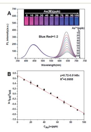
Fig. 2 (A) The fluorescent spectra of mixture of blue CDs and red QD chains at ratios 1:2 with the addition of As(III). The insets show the corresponding fluorescent photo under 365 nm UV lamp. (B) Fluorescent intensity ratio, In ( $l_{640}/l_{445}$ ), vs. the concentrations of As(III) in the TTCA-QD chains/CDs.
