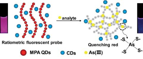
Scheme 2 Schematic illustration of the ratiometric fluorescent sensors for the detection of As(III), the insets show the corresponding fluorescent photo under 365 nm UV lamp from fushia (left) to blue (right) upon the addition of As<sup>3+</sup> in the sensing system.
