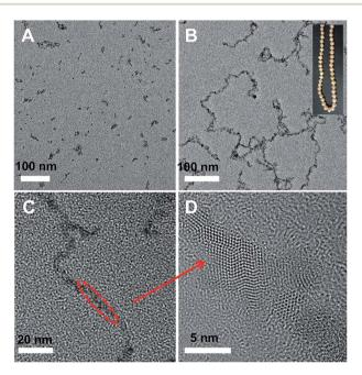
Fig. 1 TEM images of the samples. (A) CdTe QDs modified with 3mercaptopropionic acid (MPA); (B) low resolution TEM images of the TTCA-QD chains, and insert shows a photo of a chain; (C) high resolution TEM images of the TTCA-QD chains and (D) indicated structural details of the QD chains
