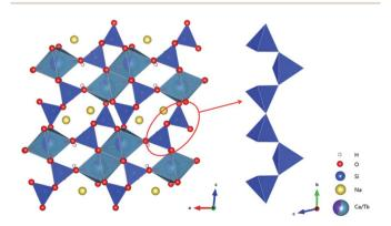
Fig. 2 Polyhedral view of the Na<sub>2</sub>Tb<sub>1.08</sub>Ca<sub>2.92</sub>Si<sub>6</sub>O<sub>18</sub>H<sub>0.8</sub> compound along the b-axis and [SiO<sub>4</sub>] tetrahedra single chain.
