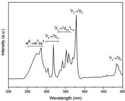
Fig. 3 Excitation spectrum of Na<sub>2</sub>Tb<sub>1.08</sub>Ca<sub>2.92</sub>Si<sub>6</sub>O<sub>18</sub>H<sub>0.8</sub> ( $\lambda_{em}=542$  nm).
