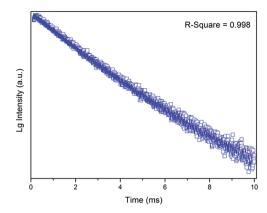
Fig. 5 RT fluorescence decay curve detected at 542 nm ( $\lambda_{em}=276$  nm). The solid line represents the best fit to the data.
