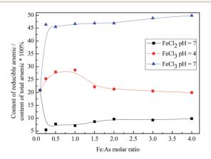
Fig. 7 The effects of the  $FeCl_2$  or  $FeCl_3$  stabilizers with different molar ratios of Fe : As on the reducible arsenic content.
