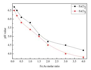
Fig. 3 The effects of the FeCl<sub>2</sub> and FeCl<sub>3</sub> stabilizers with different Fe: As molar ratios on the mixed solution pH.
