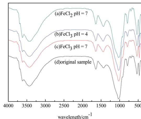
Fig. 10 The FTIR spectra of the arsenic waste slag samples obtained before and after carrying out the stabilization step using FeCl<sub>2</sub> and FeCl<sub>3</sub>.
