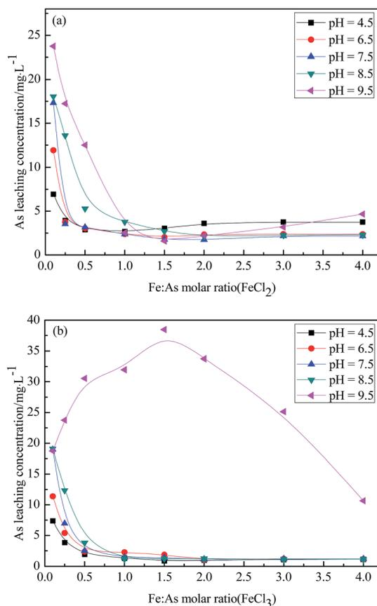
Fig. 4 The effects of the mixed solution pH with different molar ratios of Fe : As on the As leaching concentration observed using (a) FeCl<sub>2</sub> and (b) FeCl<sub>3</sub>.
