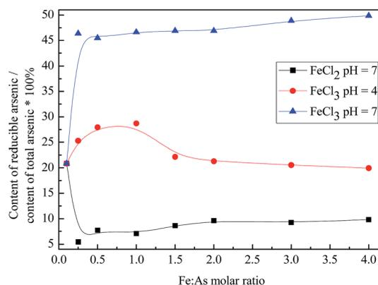
Fig. 7 The effects of the  $\text{FeCl}_2$  or  $\text{FeCl}_3$  stabilizers with different molar ratios of Fe : As on the reducible arsenic content.
