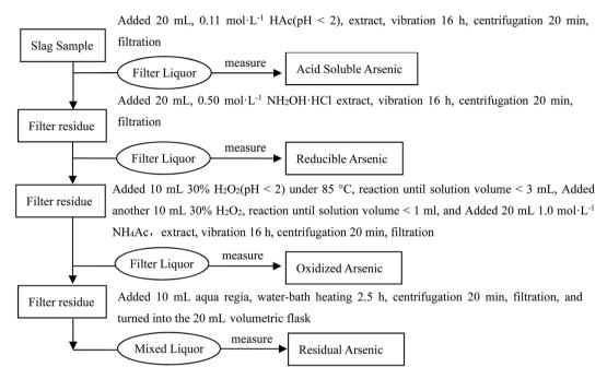
Fig. 2 The steps used in the BCR leaching extraction method.
