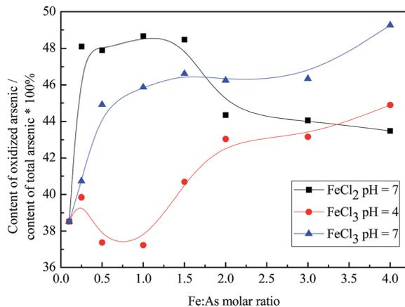
Fig. 8 The effects of the FeCl<sub>2</sub> or FeCl<sub>3</sub> stabilizers with different molar ratios of Fe : As on the oxidized arsenic content.
