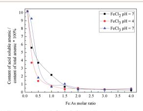
Fig. 6 The effects of the  $FeCl_2$  or  $FeCl_3$  stabilizers with different molar ratios of Fe : As on the acid-soluble arsenic content.
