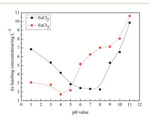
Fig. 5 The effects of the FeCl<sub>2</sub> and FeCl<sub>3</sub> stabilizers at different pH values on the As leaching concentration.
