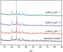
Fig. 11 The XRD spectra of the arsenic waste slag samples obtained before and after the stabilization step was carried out using FeCl<sub>2</sub> and FeCl3.
