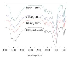
Fig. 10 The FTIR spectra of the arsenic waste slag samples obtained before and after carrying out the stabilization step using  $FeCl_2$  and  $FeCl_3$ .
