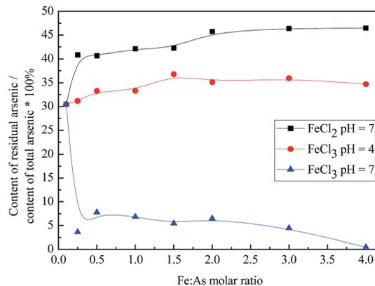
Fig. 9 The effects of the FeCl<sub>2</sub> or FeCl<sub>3</sub> stabilizers with different molar ratios of Fe : As on the residual arsenic content.
