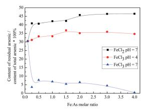
Fig. 9 The effects of the  $FeCl_2$  or  $FeCl_3$  stabilizers with different molar ratios of Fe : As on the residual arsenic content.
