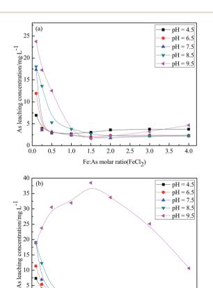
Fig. 4 The effects of the mixed solution pH with different molar ratios of Fe: As on the As leaching concentration observed using (a) FeCl<sub>2</sub> and (b) FeCl3.
