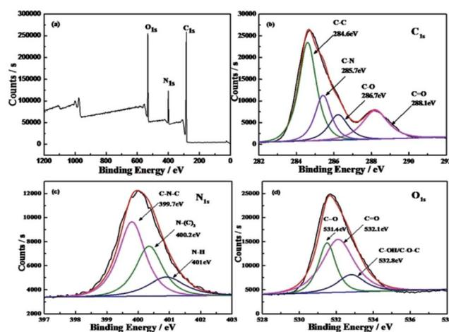
Fig. 2 XPS survey scan of the as-prepared CDs. (a) Survey, high resolution N<sub>1s</sub> (b), C<sub>1s</sub> (c), and O<sub>1s</sub> (d) XPS spectra of CDs.
