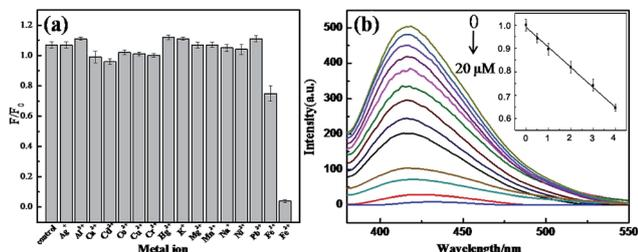
Fig. 5 Investigation of the sensitivity and selectivity in  $\text{Fe}^{3+}$  detection. (a) The influence of metal ions on the fluorescence intensity of the CDs. The concentration of metal ions was  $125 \mu\text{M L}^{-1}$ . (b) The fluorescence intensity of the CDs varied with the  $\text{Fe}^{3+}$  concentration, and the concentration of  $\text{Fe}^{3+}$  was in the range from 0 to 20  $\mu\text{M}$ . The inset figure shows the linear relationship from 0.5 to 4  $\mu\text{M}$ .
