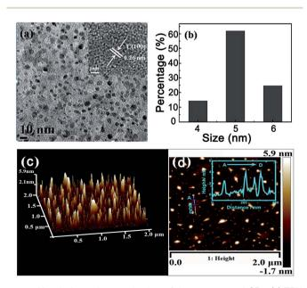
Fig. 1 Morphology characterization of the as-prepared CDs. (a) TEM image of CDs, (b) statistical distribution of the sizes of the CDs, (c) three-dimensional AFM image of the CDs, and (d) AFM image; inset: height distribution of the CDs.
