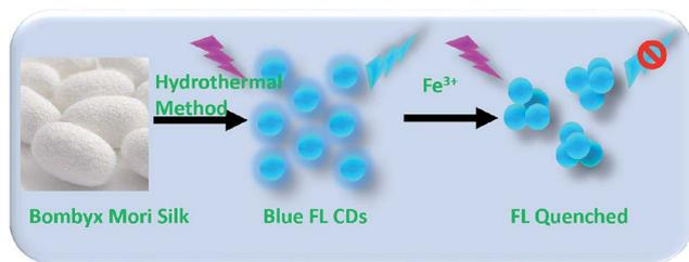
**Scheme 1** Illustration of the formation process of highly luminescent nitrogen-doped CDs with blue FL and its further applications for  $\text{Fe}^{3+}$  detection. Using *Bombyx mori* silk and citric acid as raw materials, nitrogen-doped CDs with blue FL were prepared *via* hydrothermal method. Hydroxyl groups on the surface of the CDs can interact with  $\text{Fe}^{3+}$  which induces the aggregation of CDs, resulting in FL quenching of CDs.
