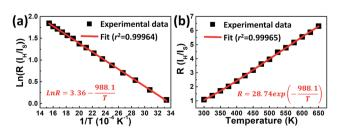
Fig. 3 (a) Monolog plot of the FIR of the green UC emissions for the  ${}^2H_{11/2}/{}^4S_{3/2} \rightarrow {}^4I_{15/2}$  transitions as a function of the inverse absolute temperature. (b) FIR of the green UC emissions for the  ${}^2H_{11/2}/{}^4S_{3/2} \rightarrow {}^4I_{15/2}$  transitions relative to the temperature.
