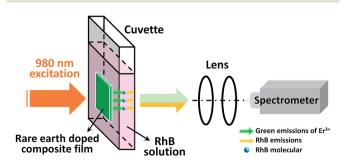
Fig. 5 Schematic diagram of the luminescence measurement of the RhB concentration-dependent UC emissions.
