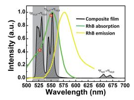
Fig. 6 UC emission spectrum of the Ag/ZnO/Er $^{3+}$ :YbMoO $_4$  composite film (black line) under the measurement condition in Fig. 5. The normalized RhB absorption (green line) and emission (yellow line) spectra are presented for comparison. The asterisks calculated by eqn (6) denote the relative RhB absorption coefficients of the two green UC emissions for the  $^2$ H $_{11/2}/^4$ S $_{3/2}$   $\rightarrow$   $^4$ I $_{15/2}$  transitions.
