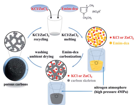
Fig. 1 Schematic showing the preparation process of the porous carbon monolith.
