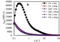
Fig. 5 Influence of shear rate on apparent viscosities of an aqueous 2.0 g  $L^{-1}$  PASV solution (a) and of a 2.0 g  $L^{-1}$  PASV brine solution with 70 g  $L^{-1}$  NaCl (b) at atmospheric pressure and 30 °C.
