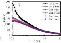
Fig. 6 Influence of shear rate on the apparent viscosities of an aqueous 2.0 g  $L^{-1}$  HPAM solution (a) and of a 2.0 g  $L^{-1}$  HPAM brine solution with 70 g  $L^{-1}$  NaCl (b) at atmospheric pressure and 30 °C.
