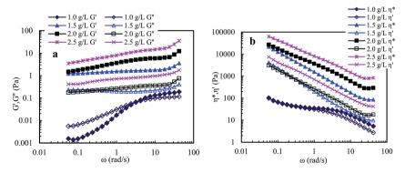
Fig. 9 Influence of angular frequency on elastic modulus G' and viscous modulus G' (a), and on dynamic viscosity  $\eta'$  and complex viscosity  $\eta^*$  (b) for PASV brine solutions with different polymer concentrations. NaCl concentration: 70 g  $L^{-1}$ .
