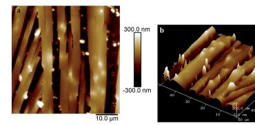
Fig. 2 AFM images of the film made using an aqueous 0.5 g L<sup>-1</sup> PASV solution. (a) Planar morphology; (b) three-dimensional morphology.
