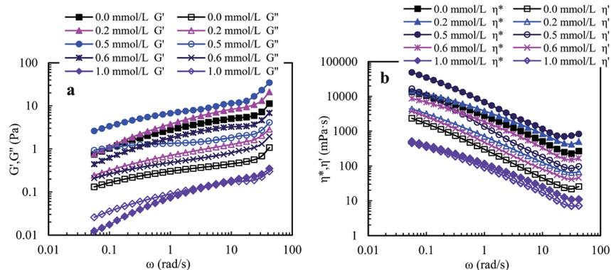
Fig. 12 Influence of angular frequency on elastic modulus  $G'$  and viscous modulus  $G''$  (a), and on dynamic viscosity  $\eta'$  and complex viscosity  $\eta^*$  (b) for aqueous  $2.0 \text{ g L}^{-1}$  PASV solutions with different SDBS concentrations.
