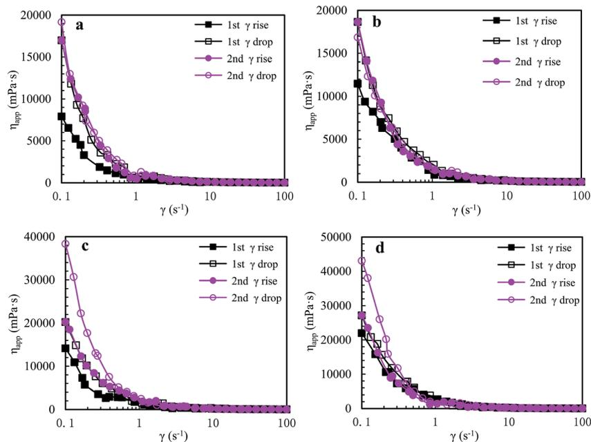
Fig. 7 Influence of shear rate on apparent viscosities of a 2.0 g L<sup>-1</sup> PASV brine solution with 70 g L<sup>-1</sup> NaCl at different pressures and 65 °C. (a) 0 MPa; (b) 10 MPa; (c) 15 MPa; and (d) 20 MPa.
