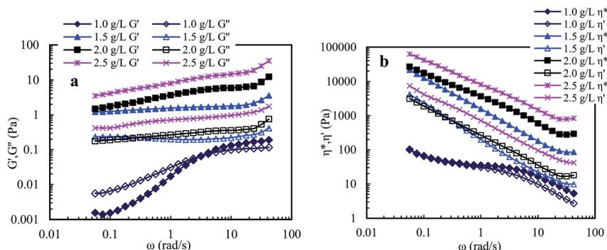
Fig. 9 Influence of angular frequency on elastic modulus  $G'$  and viscous modulus  $G''$  (a), and on dynamic viscosity  $\eta'$  and complex viscosity  $\eta^*$  (b) for PASV brine solutions with different polymer concentrations. NaCl concentration:  $70 \text{ g L}^{-1}$ .
