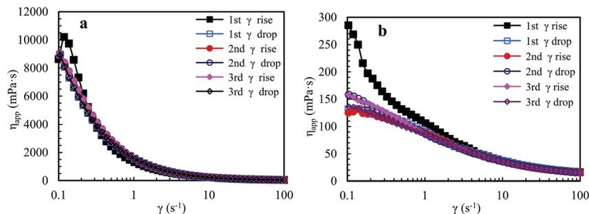
Fig. 6 Influence of shear rate on the apparent viscosities of an aqueous  $2.0 \text{ g L}^{-1}$  HPAM solution (a) and of a  $2.0 \text{ g L}^{-1}$  HPAM brine solution with  $70 \text{ g L}^{-1}$  NaCl (b) at atmospheric pressure and  $30 \text{ }^\circ\text{C}$ .
