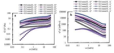
Fig. 13 Influence of angular frequency on elastic modulus G' and viscous modulus G'' (a), and on dynamic viscosity  $\eta'$  and complex viscosity  $\eta^*$ (b) of 2.0 g  $L^{-1}$  PASV brine solutions with different SDBS concentrations. NaCl concentration: 70 g  $L^{-1}$ .
