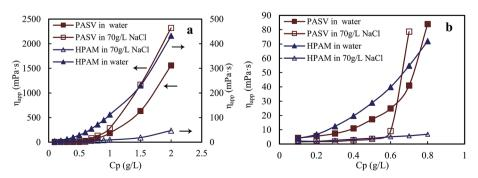
Fig. 1 Effect of polymer concentration on apparent viscosities of aqueous and brine solutions. (a) Polymer concentration: 0.1–2.0 g L<sup>-1</sup>; (b) polymer concentration:  $0.1-0.8 \text{ g L}^{-1}$ .
