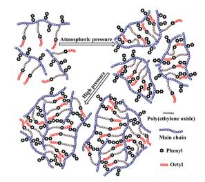
Scheme 4 Schematic structure of pressure-thickening for PASV.
