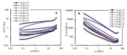
Fig. 8 Influence of angular frequency on elastic modulus G' and viscous modulus G' (a), and on dynamic viscosity  $\eta'$  and complex viscosity  $\eta^*$  (b) for aqueous PASV solutions with different polymer concentrations.
