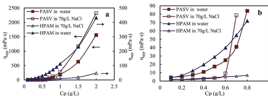
Fig. 1 Effect of polymer concentration on apparent viscosities of aqueous and brine solutions. (a) Polymer concentration: 0.1–2.0  $\text{g L}^{-1}$ ; (b) polymer concentration: 0.1–0.8  $\text{g L}^{-1}$ .
