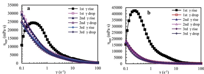
Fig. 5 Influence of shear rate on apparent viscosities of an aqueous  $2.0 \text{ g L}^{-1}$  PASV solution (a) and of a  $2.0 \text{ g L}^{-1}$  PASV brine solution with  $70 \text{ g L}^{-1}$  NaCl (b) at atmospheric pressure and  $30 \text{ }^\circ\text{C}$ .
