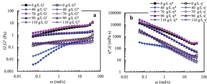
Fig. 10 Influence of angular frequency on elastic modulus  $G'$  and viscous modulus  $G''$  (a), and on dynamic viscosity  $\eta'$  and complex viscosity  $\eta^*$  (b) for  $2.0 \text{ g L}^{-1}$  PASV brine solutions with different NaCl concentrations.
