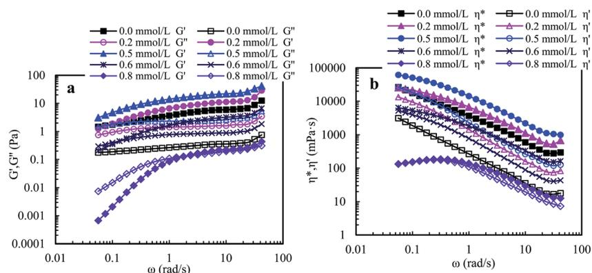
Fig. 13 Influence of angular frequency on elastic modulus  $G'$  and viscous modulus  $G''$  (a), and on dynamic viscosity  $\eta'$  and complex viscosity  $\eta^*$  (b) of  $2.0 \text{ g L}^{-1}$  PASV brine solutions with different SDBS concentrations. NaCl concentration:  $70 \text{ g L}^{-1}$ .
