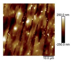
Fig. 3  $\,$  AFM image of the film made using an aqueous 0.7 g L $^{-1}$  PASV solution.
