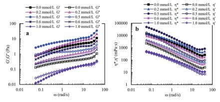
Fig. 12 Influence of angular frequency on elastic modulus G' and viscous modulus G'' (a), and on dynamic viscosity  $\eta'$  and complex viscosity  $\eta^*$ (b) for aqueous 2.0 g  $\rm L^{-1}$  PASV solutions with different SDBS concentrations.
