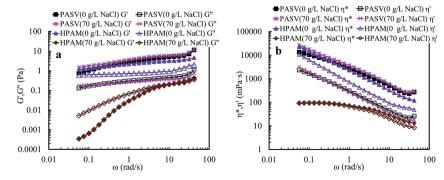
Fig. 11 Influence of angular frequency on elastic modulus G' and viscous modulus G'' (a), and on dynamic viscosity  $\eta'$  and complex viscosity  $\eta^*$  (b) for PASV and HPAM in aqueous and 70 g L<sup>-1</sup> NaCl solutions. Polymer concentration: 2.0 g L<sup>-1</sup>.
