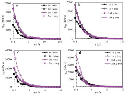
Fig. 7 Influence of shear rate on apparent viscosities of a 2.0 g  $L^{-1}$  PASV brine solution with 70 g  $L^{-1}$  NaCl at different pressures and 65 °C. (a) 0 MPa; (b) 10 MPa; (c) 15 MPa; and (d) 20 MPa.
