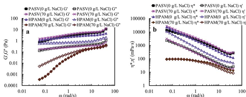
Fig. 11 Influence of angular frequency on elastic modulus  $G'$  and viscous modulus  $G''$  (a), and on dynamic viscosity  $\eta'$  and complex viscosity  $\eta^*$  (b) for PASV and HPAM in aqueous and  $70 \text{ g L}^{-1}$  NaCl solutions. Polymer concentration:  $2.0 \text{ g L}^{-1}$ .
