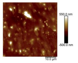
Fig. 4  $\,$  AFM image of the film made using an aqueous 1.0 g  $\rm L^{-1}$  PASV solution.
