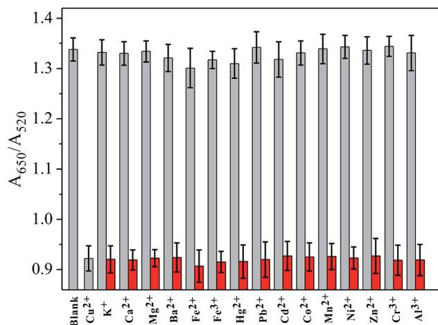
**Fig. 4** Absorbance ratios of PEG-AuNPs when different kinds of foreign ions were added alone and along with  $\text{Cu}^{2+}$ . Gray bars represent the addition of single metal ion; red bars are the addition of  $\text{Cu}^{2+}$  with another metal ion. The concentration of  $\text{Cu}^{2+}$  was 250 nM, and other metal ions were all 5.0  $\mu\text{M}$ .
