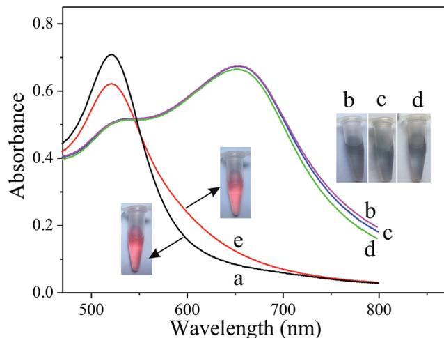
**Fig. 1** UV-vis spectra of (a) PEG-AuNPs, (b) PEG-AuNPs + cysteine (25  $\mu\text{M}$ ), PEG-AuNPs containing the mixtures of (c) cysteine (25  $\mu\text{M}$ ) +  $\text{Cu}^{2+}$  (2  $\mu\text{M}$ ), (d) cysteine (25  $\mu\text{M}$ ) +  $\text{H}_2\text{O}_2$  (1 mM) and (e) cysteine (25  $\mu\text{M}$ ) +  $\text{H}_2\text{O}_2$  (1 mM) +  $\text{Cu}^{2+}$  (2  $\mu\text{M}$ ). The inset photographic images are the corresponding colorimetric response.
