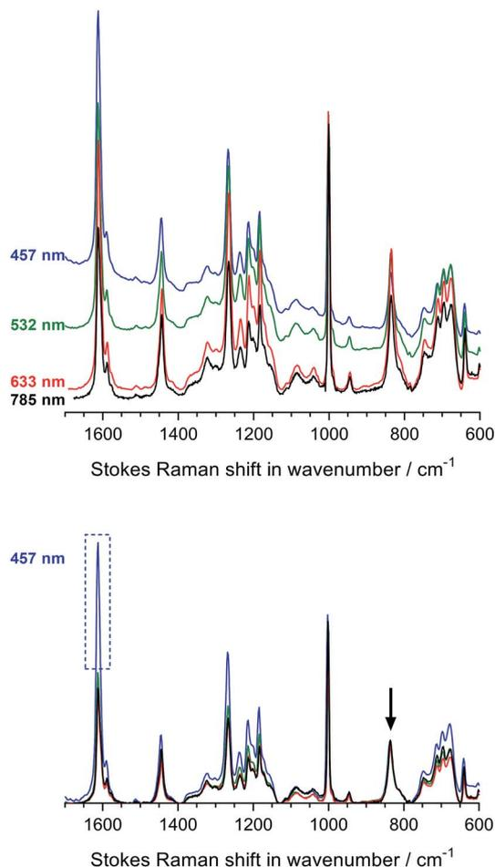
Fig. 3 The Raman spectra of **Int16** both with (bottom graph) and without (top graph) baseline correction and normalisation. The baseline-corrected spectra were normalised to the intensity of the CF<sub>2</sub> stretch peak at 835 cm<sup>-1</sup> peak to aid visual comparison (the peak indicated by arrow). The enhancement in the 1612 cm<sup>-1</sup> peak when using the 457 nm laser is shown by the dashed box.
