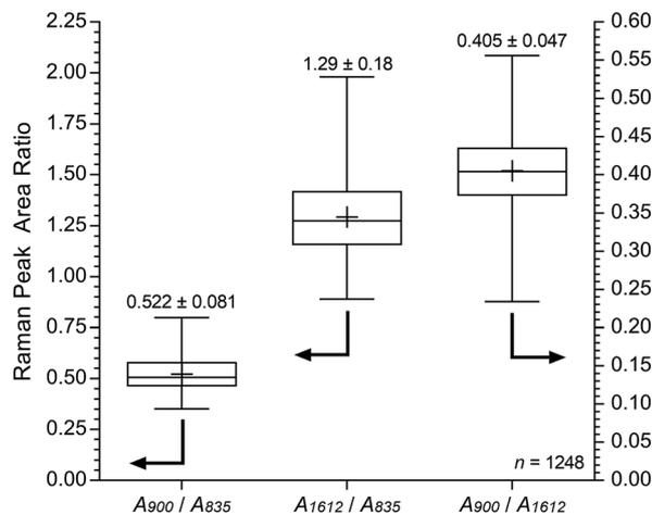
Fig. 9 Box and whisker plot summarising the cross-sectional Raman spectral data (785 nm laser) for **E16** (extracted from Fig. 8). The + symbols give the means, the middle horizontal lines give the medians, the boxes give the interquartile ranges, and the whiskers give the min and max values recorded. The numeric data presented gives the mean and sample standard deviations ( $n = 1248$ ).
