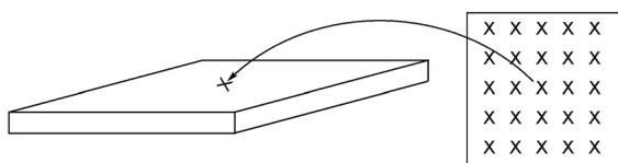
Fig. 10 A diagram showing the sampling of the Raman spectra recorded on the surfaces of **E16** and **AE16** (ca.  $1 \text{ cm}^2$  samples in this study).
