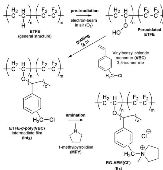
**Scheme 1** An outline of the synthesis of ETFE-based pyrrolidinium-type radiation-grafted anion-exchange membranes (RG-AEM) in the chloride-anion form. The precursor ETFE film used in this study was 50 μm thick. The main variable in this study was the grafting time (x).
