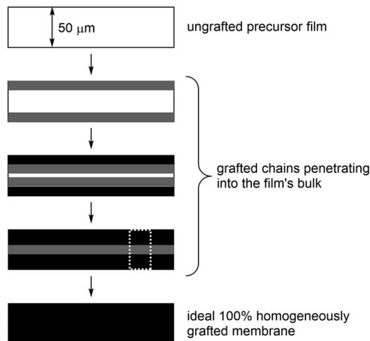
Fig. 1 A diagram showing the grafting front mechanism that is commonly encountered in the synthesis of radiation-grafted membranes. The white dashed rectangle indicates a typical Raman spectro-microscopy cross-sectional mapping region (*i.e.* the  $30 \times 65 \mu\text{m}$  areas used in this study).
