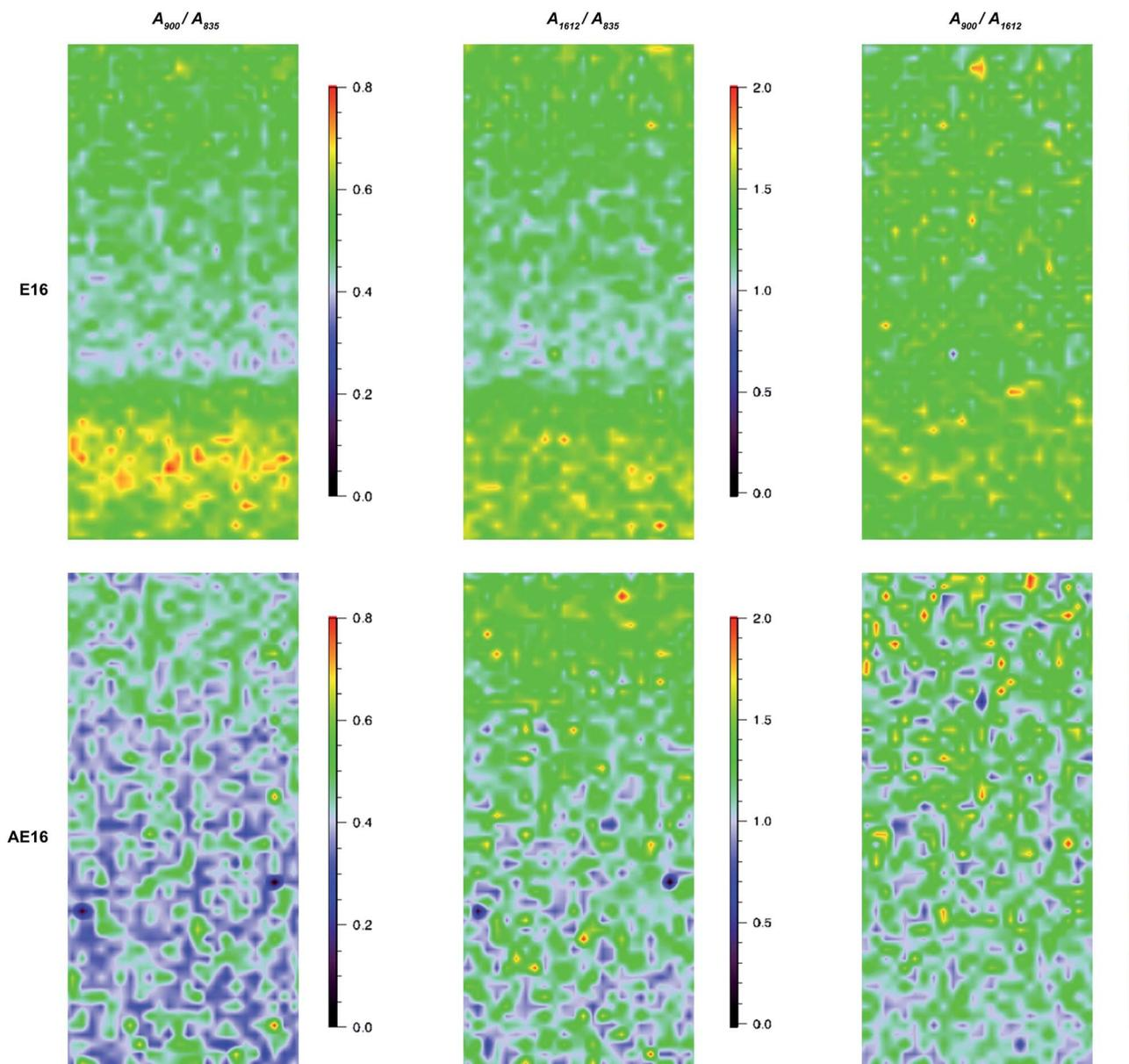
Fig. 8 Raman cross-sectional interpolated maps of **E16** (top row) and **AE16** (bottom row) recorded using the 785 nm laser (300 mW power, pinhole applied) with par-sampling. The colour scale represents (from left to right columns):  $A_{900}/A_{835}$  (pyrrolidinium vs. ETFE);  $A_{1612}/A_{835}$  (benzene vs. ETFE);  $A_{900}/A_{1612}$  (pyrrolidinium vs. benzene). Each map is  $30 \times 65 \mu\text{m}$  in size ( $y$ -axis is the through-plane direction).
