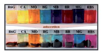
Fig. 7 Photographs of different dye solutions before and after adsorption by the GO/SA/PAM composite hydrogels.  $^{65}$
