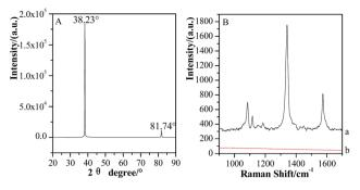
Fig. 4 XRD characterization of the GSCPs (A) and SERS spectra of 1 mmol  $L^{-1}$  of pNTP adsorbed on GSCPs with (a) or without (b) Au@SiO<sub>2</sub> SHINs (B).
