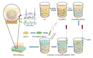
Scheme 1 The principle of self-assembly of (Au-pMBA)@ $SiO_2$  film on TP-modified GSCP substrate.
