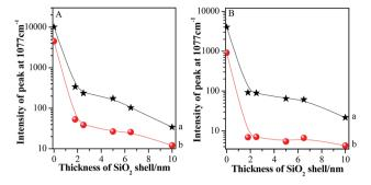
**Fig. 6** The relationships between silica shell thicknesses and absolute SERS peak intensities of pMBA at 1077 cm<sup>-1</sup> using 633 nm (A) or 785 nm (B) illumination as excitation wavelength ((a): GSCPs area; (b): beyond the area of GSCPs).
