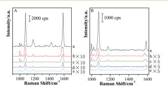
Fig. 8 SERS spectra of (Au-pMBA)@SiO $_2$  films of various silica thicknesses: 0 nm (a), 1.8 nm (b), 2.5 nm (c), 5 nm (d) and 6.5 nm (e) covering on TP-modified GSCPs using 633 nm (A) or 785 nm (B) illumination as excitation wavelength.
