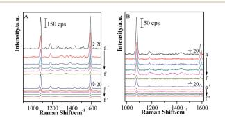
Fig. 5 SERS spectra of (Au-pMBA)@SiO $_2$  films of various silica shell thicknesses: 0 nm (a, a'), 1.8 nm (b, b'), 2.5 nm (c, c'), 5 nm (d, d'), 6.5 nm (e, e') and 10 nm (f, f') in the areas of (a  $\rightarrow$  f) and beyond (a'  $\rightarrow$  f') GSCPs using 633 nm (A) or 785 nm (B) illumination as excitation wavelength.
