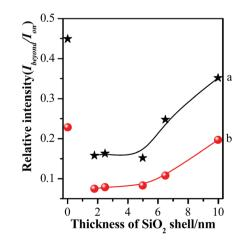
Fig. 7 Comparison of relative SERS intensities  $(I_{\rm beyond}/I_{\rm on})$  of various silica shell thicknesses using 633 nm (a) or 785 nm (b) illumination as excitation wavelength.
