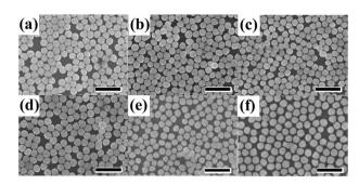
Fig. 2 SEM images of (Au-pMBA)@SiO $_2$  films with the silica shell thicknesses of about 0 nm (a), 1.8 nm (b), 2.5 nm (c), 5 nm (d), 6.5 nm (e) and 10 nm (f). Scale bar: 500 nm.
