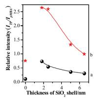
Fig. 10 The relationships between silica shell thicknesses and relative SERS peak intensities ( $I_{\rm TP}/I_{\rm pMBA}$ ) using 633 nm (a) or 785 nm (b) illumination as excitation wavelength.
