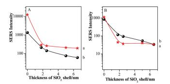
Fig. 9 The relationships between silica shell thicknesses and absolute SERS peak intensities of pMBA at about  $1588\,\mathrm{cm}^{-1}$  (a) together with TP at about  $998\,\mathrm{cm}^{-1}$  (b) using 633 nm (A) or 785 nm (B) illumination as excitation wavelength.
