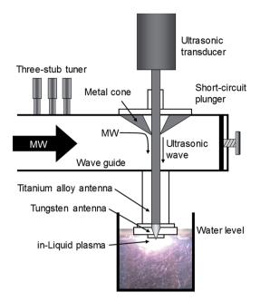
Fig. 10 Schematic diagram of an ultrasonic/microwave simultaneous irradiation type in-liquid plasma generator system. Reproduced from Horikoshi *et al.*<sup>156</sup> Copyright 2017 by Elsevier.
