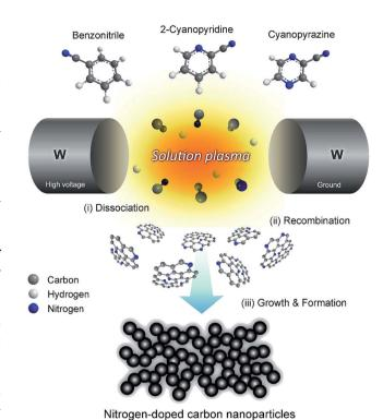
Fig. 16 Schematic illustration of the formation mechanism of nitrogen-doped carbon nanoparticles (NCNPs) *via* a solution plasma process. Modified with permission from ref. 163. Copyright 2016 by Elsevier.
