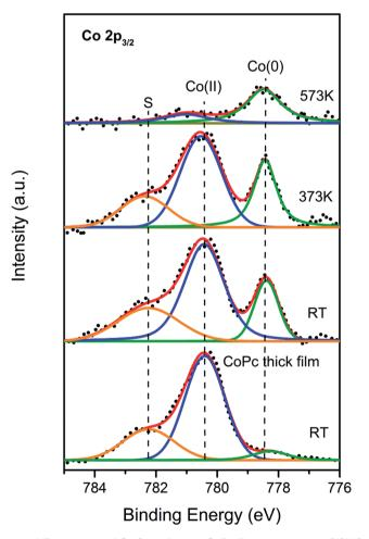
Fig. 5 XP spectrum of Co  $2p_{3/2}$  for thin CoPc film deposited on Bi(111) surface kept at RT followed by thermal annealing. Black dots: raw data; blue line: fitted Co(II) oxidation state; green line: fitted component with Co(0) state; orange line: the shake-up component associated to the Co(III) state. As a reference, a thick CoPc film was also prepared and recorded as shown in the bottom.
