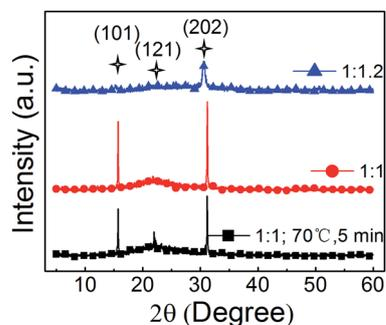
Fig. 6 The XRD patterns of three 10 wt% neat  $\text{CsPbBr}_3$  films ( $\text{PbBr}_2 : \text{CsBr} = 1 : 1$  with annealing at  $70^\circ\text{C}$  for 5 min after pumping away,  $\text{PbBr}_2 : \text{CsBr} = 1 : 1$  with just pumping away,  $\text{PbBr}_2 : \text{CsBr} = 1 : 1.2$  with just pumping away).
