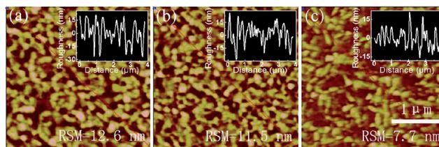
Fig. 7 AFM images for three 10 wt% neat  $\text{CsPbBr}_3$  films (a)  $\text{PbBr}_2 : \text{CsBr} = 1 : 1$  with annealing at  $70^\circ\text{C}$  for 5 min after pumping away, (b)  $\text{PbBr}_2 : \text{CsBr} = 1 : 1$  with just pumping away, (c)  $\text{PbBr}_2 : \text{CsBr} = 1 : 1.2$  with just pumping away.
