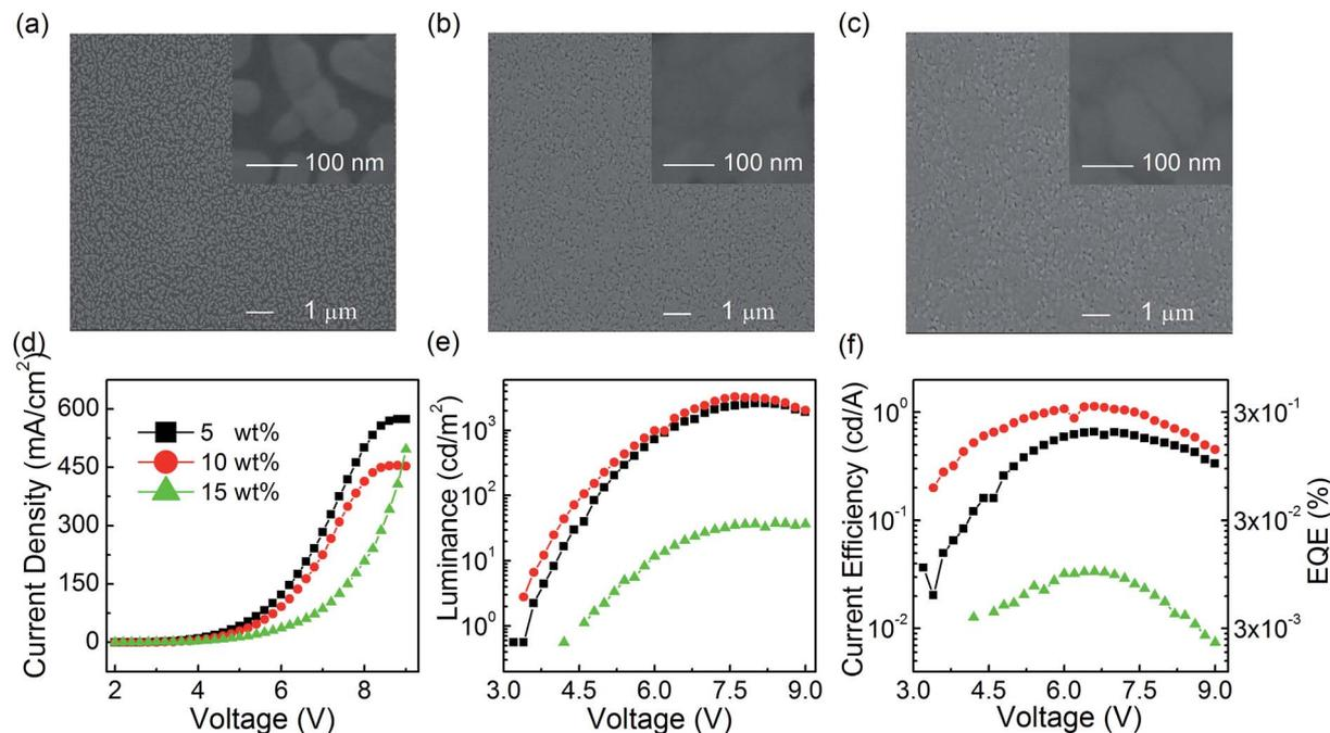
Fig. 3 The top-view SEM image of modified neat CsPbBr<sub>3</sub> film with only pumping away from different concentrations of (a) 5 wt%, (b) 10 wt%, (c) 15 wt% in DMSO precursor solution, (d)  $J$ - $V$ - $L$  relationship, (e)  $L$ - $V$  of the PeLEDs, (f) CE- $V$ -EQE relationship of the PeLEDs based on different CsPbBr<sub>3</sub> concentrations in DMSO precursor solution.
