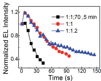
Fig. 5 The stability of PeLEDs formed by  $\text{PbBr}_2 : \text{CsBr} = 1 : 1$  with annealing at  $70^\circ\text{C}$  for 5 min after pumping away,  $\text{PbBr}_2 : \text{CsBr} = 1 : 1$  with just pumping away, and  $\text{PbBr}_2 : \text{CsBr} = 1 : 1.2$  with just pumping away.
