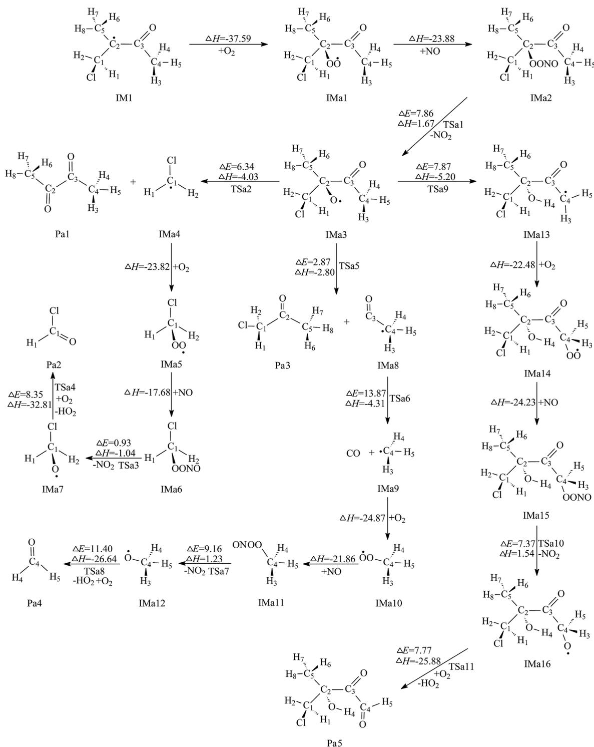
Fig. 3 Secondary reaction pathways of IM1 with the potential barriers  $\Delta E^\ddagger$  (kcal mol<sup>-1</sup>) and reaction heats  $\Delta H$  (kcal mol<sup>-1</sup>).
