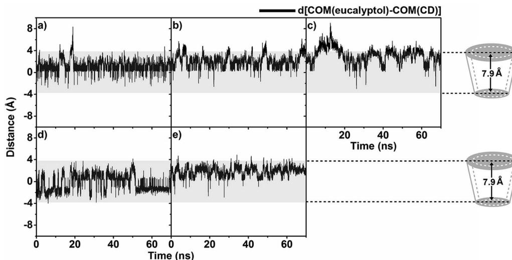
Fig. 4 Distances between centers of mass of eucalyptol and CD molecules in (a) eucalyptol/ $\beta$ CD, (b) eucalyptol/2,6-DM $\beta$ CD, (c) eucalyptol/2-HP $\beta$ CD, (d) eucalyptol/6-HP $\beta$ CD and (e) eucalyptol/2,6-DHP $\beta$ CD inclusion complexes.
