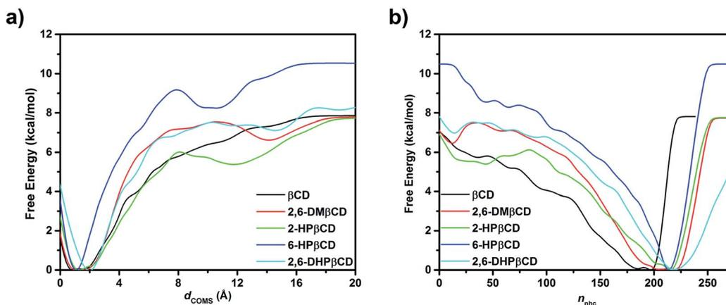
Fig. 6 Free energy profiles resulting from metadynamics of eucalyptol dissociation from  $\beta$ CD cavity and each of its derivative along (a) CV1, distance between centers of mass of eucalyptol and CDs ( $d_{COMS}$ ) and (b) CV2, number of hydrophobic contacts ( $n_{nhc}$ ) between non-polar carbons of eucalyptol and CDs.
