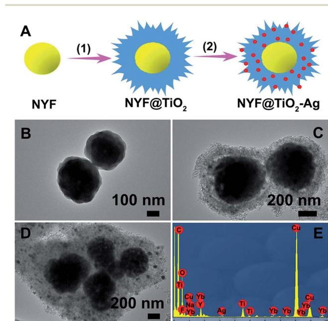
Fig. 1 (A) Schematic illustration of the synthesis process of the NYF@TiO<sub>2</sub>-Ag core-shell microspheres. TEM images of (B) NYF, (C) NYF@TiO<sub>2</sub>, (D) NYF@TiO<sub>2</sub>-2 wt% Ag photocatalyst. (E) The EDX spectrum of the NYF@TiO<sub>2</sub>-2 wt% Ag photocatalyst.
