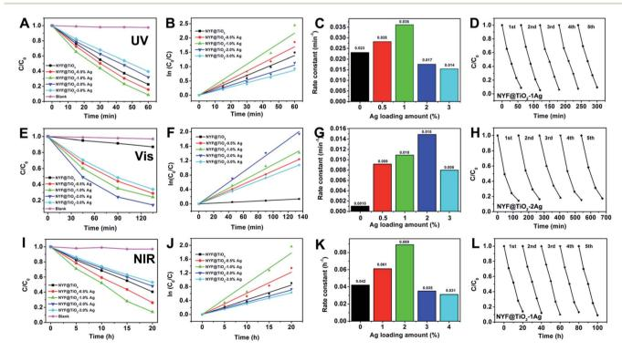
Fig. 3 Photocatalytic degradation of MO aqueous solution in the present of the NYF@TiO $_2$ -x wt% Ag (x = 0, 0.5, 1, 2, and 3) photocatalysts under (A-D) UV, (E-H) visible (I-L) NIR light irradiation. The plot of  $(C/C_0)$  vs. reaction time (A, E, I),  $\ln(C_0/C)$  vs. reaction time (B, F, J), the apparent rate constants vs. Ag loading (C, G, K), photocatalytic stability in five successive cycling reactions (D, H, L).
