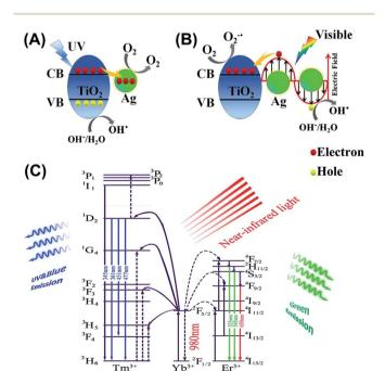
Fig. 5 Proposed photocatalytic mechanism of NYF@TiO $_2$ -Ag photocatalyst under (A) UV and (B) visible light, (C) schematic energy level diagrams, upconversion excitation and UV and visible light emissions for the NYF microspheres under the NIR light (980 nm laser) illumination.
