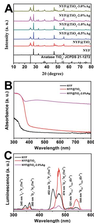
Fig. 2 (A) XRD patterns of NYF, NYF@TiO<sub>2</sub> and NYF@TiO<sub>2</sub>-*x* wt% Ag (*x* = 0, 0.5, 1, 2, and 3) samples. (B) UV-vis absorption spectra and (C) upconversion luminescence spectra of the NYF, NYF@TiO<sub>2</sub> and NYF@TiO<sub>2</sub>-2 wt% Ag samples.
