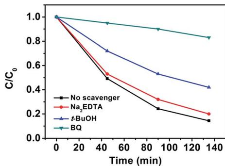
Fig. 4 Photocatalytic degradation of MO in the presence of three types of scavengers and NYF@TiO<sub>2</sub>-2 wt% Ag photocatalyst under visible light irradiation.
