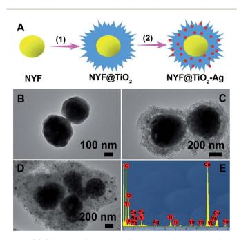
Fig. 1 (A) Schematic illustration of the synthesis process of the NYF@TiO<sub>2</sub>-Ag core@shell microspheres. TEM images of (B) NYF, (C)  $NYF@TiO_2$ , (D)  $NYF@TiO_2-2$  wt% Ag photocatalyst. (E) The EDX spectrum of the NYF@TiO2-2 wt% Ag photocatalyst.
