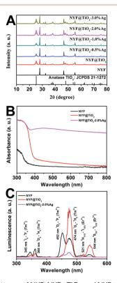
Fig. 2 (A) XRD patterns of NYF, NYF@TiO<sub>2</sub> and NYF@TiO<sub>2</sub>-x wt% Ag (x = 0, 0.5, 1, 2, and 3) samples. (B) UV-vis absorption spectra and (C) upconversion luminescence spectra of the NYF, NYF@TiO2 and NYF@TiO<sub>2</sub>-2 wt% Ag samples.
