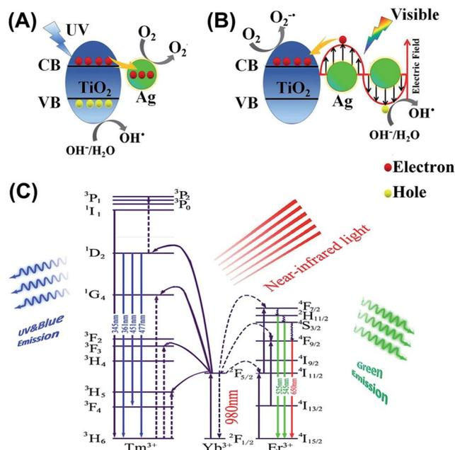
Fig. 5 Proposed photocatalytic mechanism of NYF@TiO<sub>2</sub>-Ag photocatalyst under (A) UV and (B) visible light, (C) schematic energy level diagrams, upconversion excitation and UV and visible light emissions for the NYF microspheres under the NIR light (980 nm laser) illumination.
