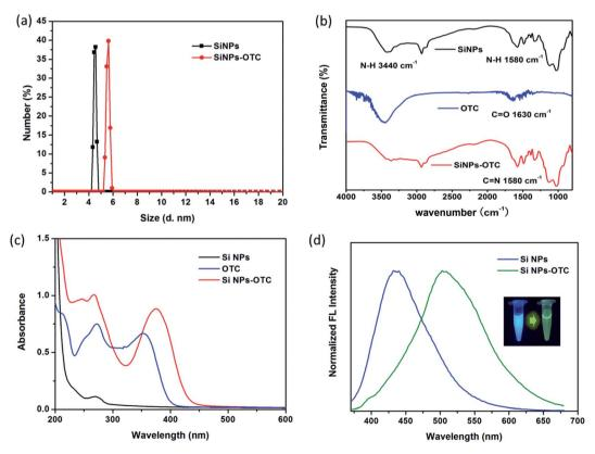
Fig. 4 (a) DLS size distribution of SiNPs and SiNPs-OTC complex through DLS measurements. (b) FT-IR and (c) absorption spectra of SiNPs (black), OTC (blue) and SiNPs-OTC complex (red). Fluorescence variation of SiNPs (blue) and SiNPs-OTC complex (green), inset is the corresponding photographs under UV lamp.
