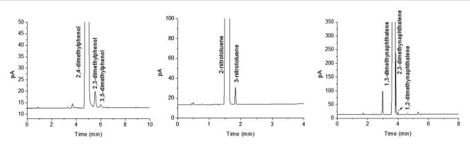
Fig. 8 Applications for the detection of isomer impurities in the commercial reagent samples on the TFTD column.
