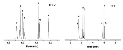
Fig. 3 GC separations of the mixture of 7 analytes on the TFTD column in comparison to the TFT column. Peaks: (1) m-cymene, (2) n-butylbenzene, (3) 1,2-dichlorobenzene, (4) 4-fluoroaniline, (5) n-hexylbenzene, (6) 1,2,3-trichlorobenzene, (7) 4-chlorophenol. Temperature program: 50 °C to 80 °C at 10 °C min<sup>-1</sup> and then 80 °C to 150 °C at 20 °C min<sup>-1</sup>, flow rate at 1.0 mL min<sup>-1</sup>.
