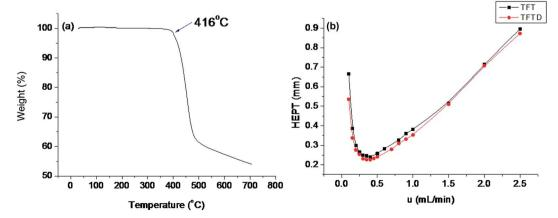
Fig. 2 (a) TGA curve of the TFTD stationary phase under nitrogen atmosphere and (b) Golay curves of the TFTD and TFT capillary columns determined by n-dodecane at 120 °C
