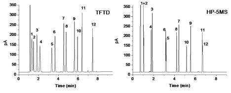
Fig. 5 GC separations of the mixture of 12 analytes on the TFTD column in comparison to the HP-5MS column. Peaks: (1) cyclohexane, (2) thiophene, (3) n-octane, (4) 1,3-dichloropropane, (5) 1-bromohexane, (6) bromobenzene, (7) n-butylbenzene, (8)1,2-dichlorobenzene, (9) 1,4-diisopropylbenzene, (10) 1,3,5-trichlorobenzene, (11) n-tridecane, (12) 1,6-dibromohexane. GC conditions: 45 °C for 1 min to 150 °C at 15 °C min<sup>-1</sup>, flow rate at 0.5 mL min<sup>-1</sup>.
