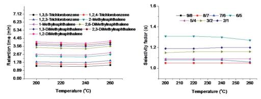
Fig. 7 Effect of conditioning temperatures on the retention times and selectivity factors of the isomers on the TFTD column. Analytes: (1) 1,3,5-trichlorobenzene, (2) 1,2,4-trichlorobenzene, (3) 1,2,3-trichlorobenzene, (4) 2-methylnaphthalene, (5) 1-methylnaphthalene, (6) 2,6-dimethylnaphthalene, (7) 1,3-dimethylnaphthalene, (8) 2,3-dimethylnaphthalene, (9) 1,2-dimethylnaphthalene.
