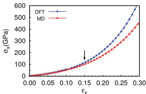
Fig. 1 The relationship between the normal pressure ( $\sigma_x$ ) and the strain ( $\epsilon_x$ ) by uniaxial compression along [100] lattice direction compared to the result of DFT method. The black arrow indicates  $\epsilon_x$  with the value of 0.15. The stress–strain curve calculated from MD method is in good agreement with that of DFT method when the strain is less than 0.15.
