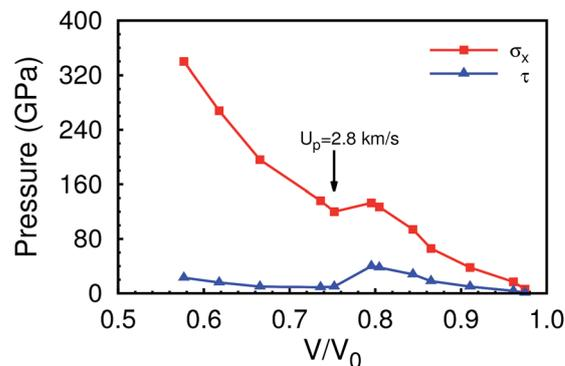
Fig. 5 The relationship between stress and volume. The maximum shear stress ( $\tau$ ) and normal pressure ( $\sigma_x$ ) along shock direction of [100] lattice direction. The black arrow indicates an inflection point at the  $V/V_0 = 0.75$  corresponding to normal pressure of 120 GPa and the piston velocity of  $2.8 \text{ km s}^{-1}$ .
