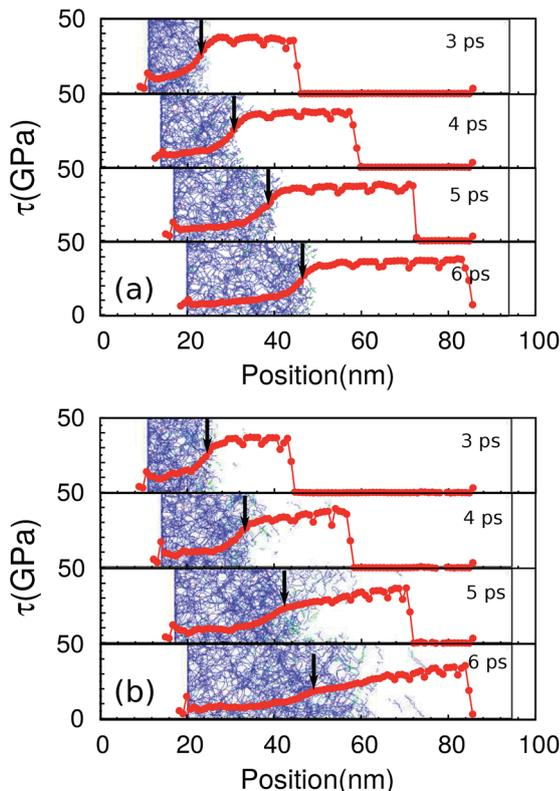
Fig. 7 The evolution of dislocation structures (blue lines) and the maximum shear stresses ( $\tau$ ) (red point line ranging from 0 to 50 GPa) in pristine MgO sample (a) and MgO single crystal with 0.1% (b). The shock front moves from left to right with the piston velocity of  $3.0 \text{ km s}^{-1}$ . The black arrows indicate the positions of plastic deformation shock front.
