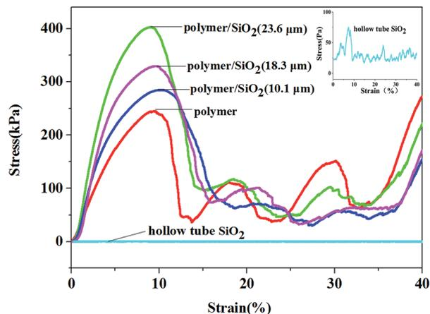
**Fig. 3** The stress–strain curves obtained for the polymer, polymer/SiO<sub>2</sub> composites, and hollow tube silica microlattices. The magnification curve obtained for the hollow tube silica microlattice is in the top right corner.
