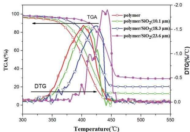
**Fig. 4** The TGA and DTG curves obtained for the polymer/SiO<sub>2</sub> composites compared with the pure polymer.
