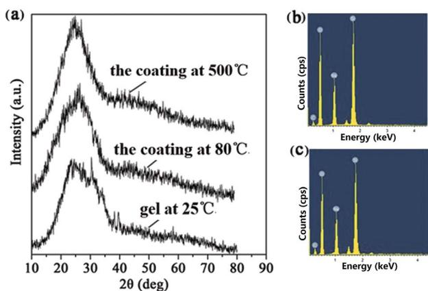
**Fig. 2** (a) The XRD patterns obtained for SiO<sub>2</sub> gel at 25 °C, the SiO<sub>2</sub> coating dried at 80 °C and the SiO<sub>2</sub> coating calcined at 500 °C. (b) The EDS patterns of the polymer/SiO<sub>2</sub> microlattices. (c) The EDS patterns of the hollow-tube SiO<sub>2</sub> microlattices.
