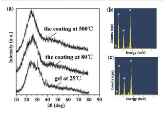
Fig. 2 (a) The XRD patterns obtained for  $SiO_2$  gel at 25 °C, the  $SiO_2$ coating dried at 80 °C and the SiO<sub>2</sub> coating calcined at 500 °C. (b) The EDS patterns of the polymer/SiO<sub>2</sub> microlattices. (c) The EDS patterns of the hollow-tube SiO<sub>2</sub> microlattices
