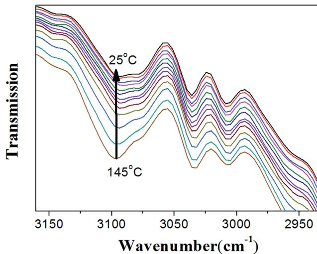
Fig. 8 *In situ* variable temperature FTIR spectra of DAER/GR-0.5 sample in the temperature range of 25–145 °C. The peaks at 3096  $\text{cm}^{-1}$ , corresponding to the signal of C=C group in the BM monomer, can be considered as the characteristic peak for the DA reactions. With decreasing the temperature from 145 °C to 25 °C, the peak intensity of 3096  $\text{cm}^{-1}$  gradually decreased, indicating the occurrence of progressive DA reaction.
