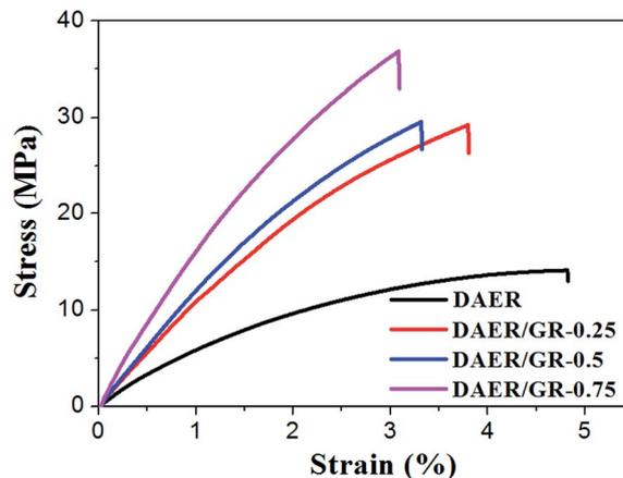
Fig. 4 Stress-strain curves of DAER and its nanocomposites measured with a strain rate of 5 mm min<sup>-1</sup> at room temperature.
