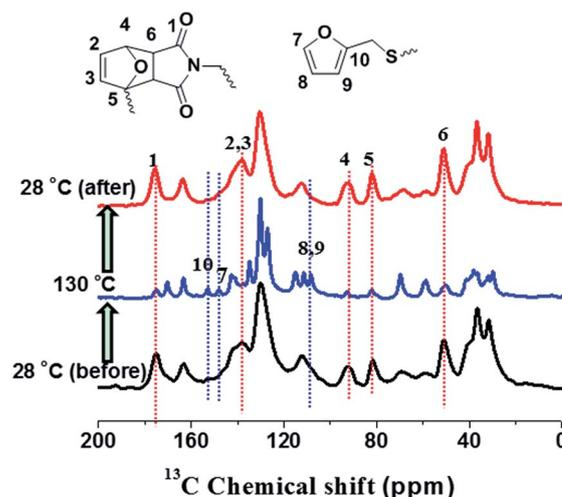
Fig. 7 *In situ* variable temperature solid-state  $^{13}\text{C}$  NMR spectra of DAER at a thermal cycle of  $28\text{ }^{\circ}\text{C}$  (black),  $130\text{ }^{\circ}\text{C}$  (blue) and  $28\text{ }^{\circ}\text{C}$  (red), respectively. The CPNOE experiment was performed to record these spectra at a NOE mixing time of 0.5 s under a MAS rate of 10 kHz.
