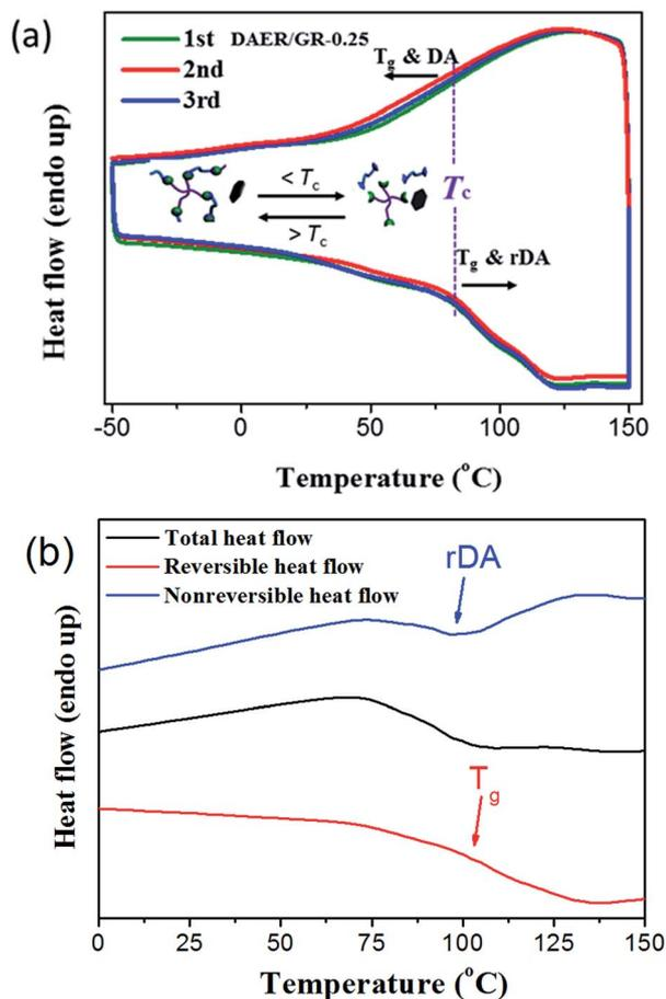
Fig. 5 (a) DSC traces of DAER/GR-0.5 in repeated cooling and heating cycles at a rate of  $10\text{ }^{\circ}\text{C min}^{-1}$ . (b) TOPEM curves of DAER/GR-0.5 sample. The heat flow for the reversible and nonreversible thermal transitions, corresponding to the glass transition and rDA reaction, are well separated, respectively. Thus, the glass transition temperature and the rDA temperature could be easily determined.
