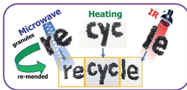
Fig. 9 Demonstration of the recyclability of DAER/GR-0.5 sample via multiple approaches, including microwave, heat and IR lights. The cracked tiny granule were put on a glass plate, and then irradiated with microwave, IR or heating without any other further manipulation.
