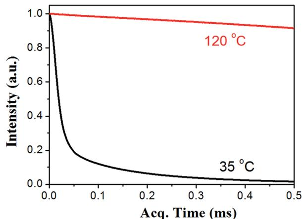
Fig. 6 The MSE-FID signals of DAER/GR-0.5 sample recorded at a temperature of  $35\text{ }^{\circ}\text{C}$  and  $120\text{ }^{\circ}\text{C}$ , respectively. At the low temperature, the sample is quite rigid, resulting in fast proton signal decay within tens of microsecond. In contrast, at a high temperature, the ER network is dissociated, and the sample becomes liquid, leading to extremely slow signal decay.
