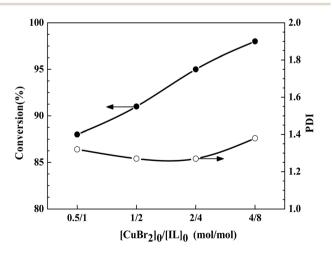
Fig. 5 Dependence of conversion and PDI on the molar ratio of  $[CuBr_2]_0/[Phmim][Ph_2PO_4]_0$  for reverse ATRP of MMA in THF. Reaction conditions:  $[MMA]_0/[AlBN]_0 = 200:1$ , MMA/THF=1:1 (v/v),  $[MMA]_0 = 9.4$  mol  $L^{-1}$ , T=70 °C.
