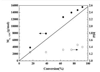
Fig. 3 Evolution of  $M_n$  (— theoretical) and PDI with monomer conversion for reverse ATRP of MMA in THF. Reaction conditions: [MMA] $_0$ /[AlBN] $_0$ /[CuBr $_2$ ] $_0$ /[Phmim][Ph $_2$ PO $_4$ ] $_0$  = 200 : 1 : 2 : 4, [MMA] $_0$  = 9.4 mol L $^{-1}$ , MMA/THF = 1 : 1 (v/v), T = 70 °C.
