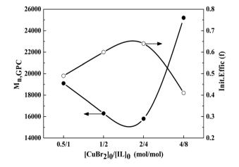
Fig. 6 Dependence of  $M_{n,GPC}$  and initiator efficiency (f) on the molar ratio of  $[CuBr_2]_0/[Phmim][Ph_2PO_4]_0$  for reverse ATRP of MMA in THF. Reaction conditions:  $[MMA]_0/[AIBN]_0 = 200:1$ , MMA/THF = 1:1 (v/v),  $[MMA]_0 = 9.4$  mol  $L^{-1}$ , T = 70 °C.
