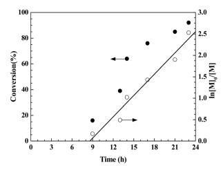
Fig. 2 Kinetic plots of  $ln([M]_0/[M])$  versus reaction time for reverse ATRP of MMA in THF. Reaction conditions:  $[MMA]_0/[AIBN]_0/[CuBr_2]_0/[Phmim][Ph_2PO_4]_0 = 200 : 1 : 2 : 4, <math>[MMA]_0 = 9.4 \text{ mol L}^{-1}$ , MMA/THF = 1 : 1 (v/v).  $T = 70 \, ^{\circ}C$ .
