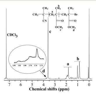
Fig. 7 <sup>1</sup>H NMR spectrum of PMMA obtained from reverse ATRP of MMA in THF. Reaction conditions: [MMA]<sub>0</sub>/[AIBN]<sub>0</sub>/[CuBr<sub>2</sub>]<sub>0</sub>/[Phmim]  $[Ph_2PO_4]_0 = 200:1:2:4$ ,  $[MMA]_0 = 9.4 \text{ mol } L^{-1}$ , MMA/THF = 1:1(v/v), reaction time = 9 h, monomer conversion = 16%, T = 70 °C.
