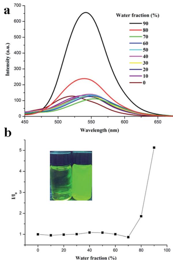
Fig. 3 (a) Fluorescence spectra of TBM in the mixtures of THF and water with different water fractions ( $f_w$ ); (b) normalized fluorescence emission intensity of TBM in THF/water with different  $f_w$ . Concentration:  $1.0 \times 10^{-5}$  M;  $\lambda_{\text{ex}} = 410$  nm; inset is the fluorescence images of TBM in THF and THF/water ( $f_w = 90\%$ ) under 365 nm illumination.
