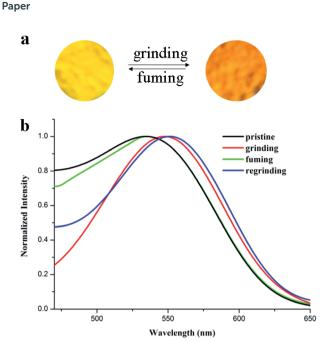
Fig. 4 (a) Photos of TBM changes under grinding and fuming stimuli; (b) normalized fluorescence spectra of TBM in different solid-states: pristine, grinding, fuming and regrinding,  $\lambda_{\rm ex} = 410$  nm.
