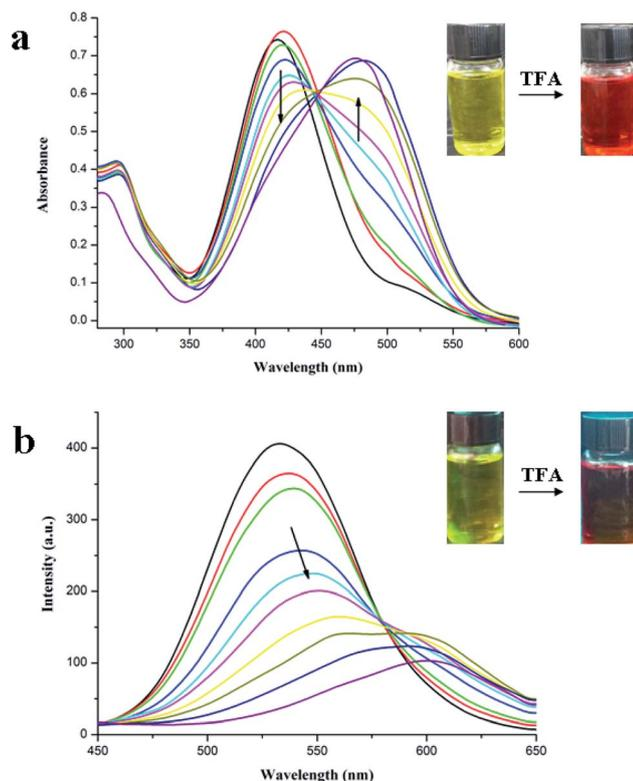
Fig. 6 (a) UV-vis absorption and (b) fluorescent emission spectral changes of **TBM** in  $\text{CHCl}_3$  from 0 equiv. to 500 equiv. with additional TFA at room temperature. The concentration of **TBM** was maintained at  $2.5 \times 10^{-5}$  M; excitation wavelength is 410 nm. Insert: images of **TBM** in  $\text{CHCl}_3$  before and after adding TFA.
