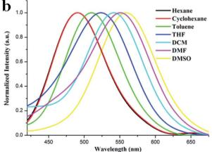
Fig. 1 Normalized UV-vis absorption (a) and fluorescent emission (b,  $\lambda_{ex}=365$  nm) spectra of TBM excited at 410 nm in different solvents (1.0  $\times$  10<sup>-5</sup> M).
