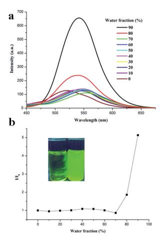
Fig. 3 (a) Fluorescence spectra of TBM in the mixtures of THF and water with different water fractions ( $f_{\rm w}$ ); (b) normalized fluorescence emission intensity of TBM in THF/water with different  $f_{\rm w}$ . Concentration:  $1.0 \times 10^{-5}$  M;  $\lambda_{\rm ex} = 410$  nm; inset is the fluorescence images of TBM in THF and THF/water ( $f_{\rm w} = 90\%$ ) under 365 nm illumination.
