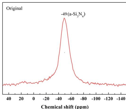
Fig. 4  $^{29}\text{Si}$  NMR spectrum of the untreated fiber.
