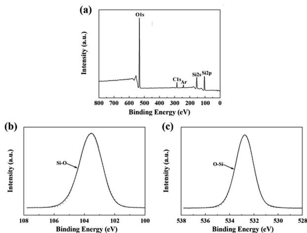
Fig. 8 XPS spectra of the fiber after the heat treatment at 1400 °C: (a) overall spectrum; (b) Si 2p; and (c) O 1s.
