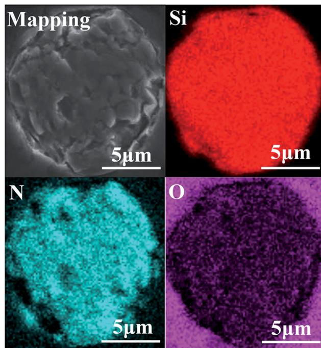
Fig. 1 Elemental distribution of the untreated fibers.
