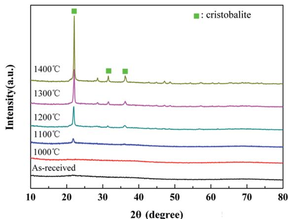
Fig. 6 XRD patterns of the untreated fibers after the heat treatment.
