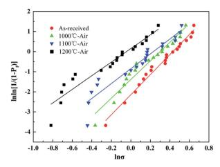
Fig. 12 Weibull plots for the fiber tested before and after the heat treatment.
