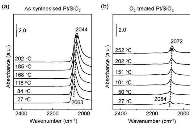
Fig. 3 Vibration frequency changes of adsorbed CO molecules on the catalyst surfaces at elevated temperature. DRIFT spectra of (a) as-synthesised and of (b) O<sub>2</sub>-treated Pt/SiO<sub>2</sub> catalysts under CO gas flow condition.
