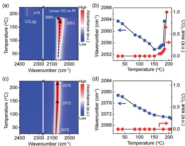
Fig. 5 Contour-maps of the *in situ* measured DRIFT spectra during the CO oxidation over Pt/SiO<sub>2</sub> catalysts and the plots of vibration frequency shifts of  $\nu(\text{C}\equiv\text{O})$  mode with integrated areas of the peaks for a  $\nu_{\text{as}}(\text{C}=\text{O})$  band. (a) A contour-map and (b) the plots for as-synthesised Pt/SiO<sub>2</sub> catalysts, and (c) a contour-map and (d) the plots for  $\text{O}_2$ -treated Pt/SiO<sub>2</sub> catalysts, respectively.
