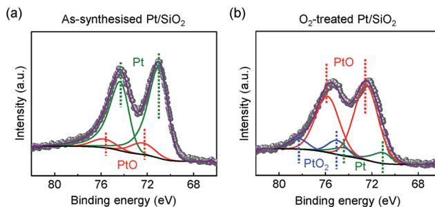
Fig. 2 XPS spectra of (a) as-synthesised and (b) O<sub>2</sub>-treated Pt/SiO<sub>2</sub> catalysts. The oxidation state of each assigned peak corresponds to metallic Pt<sup>0</sup> (green colour), Pt<sup>2+</sup> (red colour), and Pt<sup>4+</sup> (blue colour), respectively.
