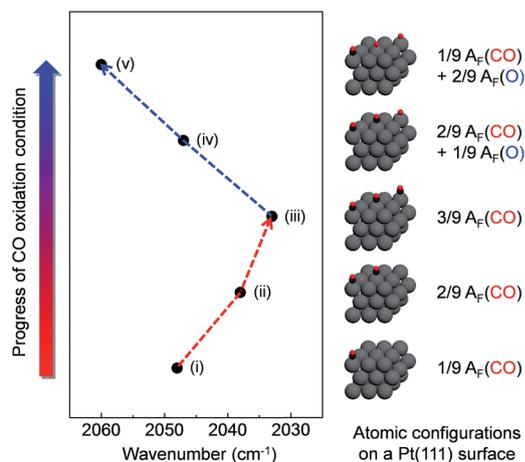
Fig. 6 Simulation results of vibration frequency shifts depending on different configurations of CO/O atomic fractions on the Pt model surface.
