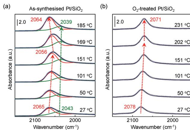
Fig. 4 DRIFT spectra of (a) as-synthesised and (b) O<sub>2</sub>-treated Pt/SiO<sub>2</sub> catalysts at elevated temperature under the mixed CO/O<sub>2</sub> gas flow condition. Deconvolution peaks correspond to vibrational modes for adsorbed CO molecules on atop sites (red colour) and on the bridge sites (green colour) of Pt atoms on a surface, respectively.
