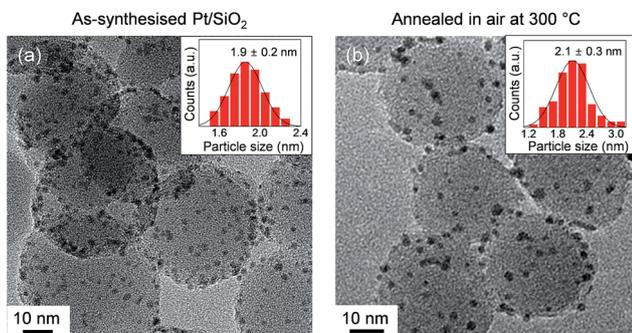
Fig. 1 TEM images and size distribution histograms of anchored Pt NPs on the spherical silica supports for (a) as-synthesised and (b) oxidised Pt/SiO<sub>2</sub> catalysts in air at 300 °C.
