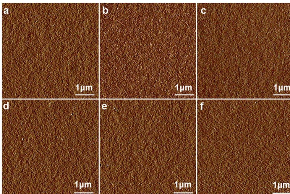
Fig. 2 AFM phase images of  $E_{C_4-2.5}$  (a),  $E_{C_8-2.5}$  (b),  $E_{C_{12}-2.5}$  (c),  $E_{C_4-5}$  (d),  $E_{C_8-5}$  (e) and  $E_{C_{12}-5}$  (f). The morphology of them was homogeneous and featureless.
