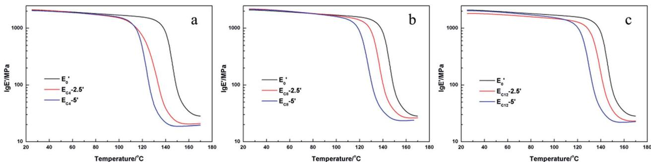
Fig. 8 Plots of storage modulus versus temperature of  $E_{C4}'$  (a),  $E_{C8}'$  (b) and  $E_{C12}'$  (c) systems.
