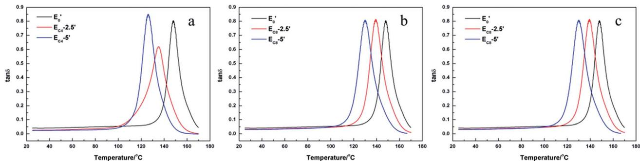
Fig. 9 Plots of loss tangent versus temperature of  $E_{C4}'$  (a),  $E_{C8}'$  (b) and  $E_{C12}'$  (c) systems.
