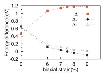
Fig. 3 Calculated electronic band gaps ( $\Delta$ ) and energy difference between the valence and conduction band valleys ( $\Delta_V$  and  $\Delta_C$ ) as a function of the applied biaxial tensile strain ranging from 0 to 9%.
