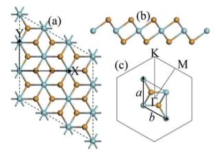
Fig. 1 (a) Top and (b) side views of monolayer  $ZrSe_2$  in  $CdI_2$  type structure, where the green and yellow balls represent the Zr and Se atoms, respectively. X and Y denote the armchair and zigzag directions of the monolayer, respectively. (c) The unit cell and corresponding Brillouin zone path with high-symmetry points at  $\Gamma(0,0,0)$ , M(0.5,0,0) and K(1/3,1/3,0).
