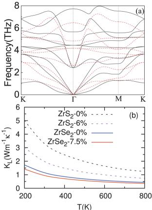
Fig. 5 (a) Calculated phonon dispersion under 0% (denoted by the black solid line) and 7.5% (denoted by the dashed line) strain. (b) Lattice thermal conductivity comparison of ZrS<sub>2</sub> (under 0% and 6% strain) and ZrSe<sub>2</sub> (under 0% and 7.5% strain) monolayers from 200 K to 800 K.
