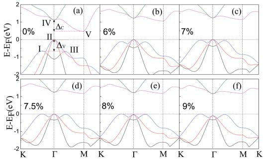
Fig. 2 Band structures of the ZrSe<sub>2</sub> monolayer along high-symmetry k-points under different biaxial strains of (a) 0%, (b) 6%, (c) 7%, (d) 7.5%, (e) 8%, and (f) 9%. The three valence band valleys near the Fermi level are denoted by I, II, and III, respectively. The two conduction band valleys near the Fermi level are denoted by IV and V, respectively.  $\Delta_V$  ( $\Delta_C$ ) represents the energy difference between I and II (IV and V).
