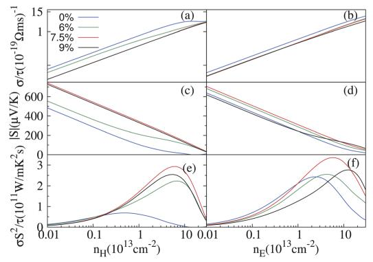
Fig. 4 Calculated transport coefficients  $\sigma/\tau$  (a and b), S (c and d), and  $\sigma/S^2\tau$  (e and f) under different biaxial strains of 6%, 7.5% and 9% as a function of carrier concentration. The left and right panels correspond to p- and n-type doping at room temperature, respectively.
