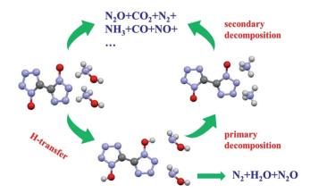
Fig. 14 The proposed thermal decomposition mechanism of TKX-50.
