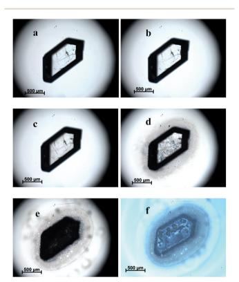
Fig. 1 The morphological changes of TKX-50 under heat stimulation. (a) The morphology of TKX-50 at 30 °C; (b) the morphology of TKX-50 at 175 °C; (c) the morphology of TKX-50 when the temperature has just risen to 198 °C; (d) the morphology of TKX-50 when the temperature has risen to 198 °C and been maintained for 1 hour; (e) the morphology of TKX-50 after primary decomposition; (f) the morphology of TKX-50 after primary decomposition using the reflection mode of the microscope.
