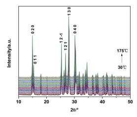
Fig. 2 XRD patterns of TKX-50 with increasing temperature from 30 to 175  $^{\circ}$ C.
