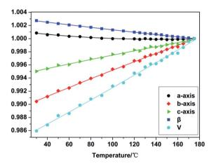
Fig. 3 Calculated unit cell parameters of TKX-50 normalized from 30 to 175  $^{\circ}$ C.
