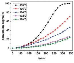
Fig. 5 Conversion degree of TKX-50 to the intermediate product at different isothermal temperatures.
