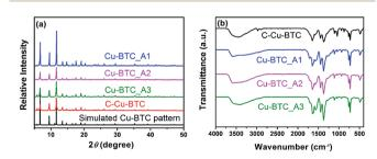
Fig. 1 (a) Powder XRD patterns of C-Cu-BTC and Cu-BTC\_An (n = 1, 2, 3) synthesized from solutions containing various molar concentrations of organic amine, and the simulated Cu-BTC XRD pattern; (b) FTIR spectra of the as-synthesized Cu-BTC\_An (n = 1, 2, 3) and C-Cu-BTC samples
