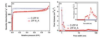
Fig. 6 (a)  $\rm N_2$  adsorption–desorption isotherms and (b) pore size distributions of ZIF-8\_A and C-ZIF-8.
