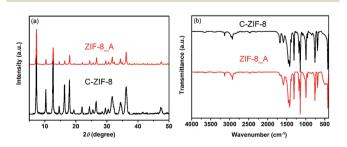
Fig. 5 (a) Powder XRD patterns of ZIF-8\_A and C-ZIF-8; (b) FTIR spectra of ZIF-8\_A and C-ZIF-8.
