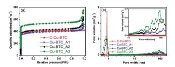
Fig. 3 (a)  $N_2$  adsorption—desorption isotherms and (b) pore size distributions (PSD) of the hierarchical porous  $Cu-BTC\_An$  (n=1, 2, 3) samples. For show the line shapes more clearly, the isotherms of  $Cu-BTC\_A2$  and  $Cu-BTC\_A3$  are vertically offset by 20 and 120 cm<sup>3</sup> g<sup>-1</sup>, respectively.
