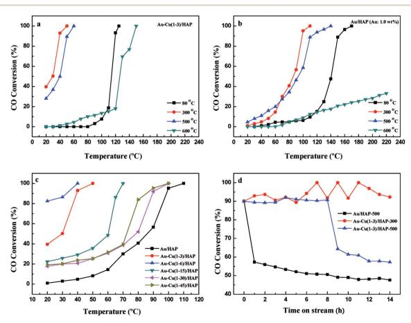
Fig. 12 Catalytic activity of Au-Cu(1-3)/HAP (Au: 1.0 wt%) (a) and Au/HAP (Au: 1.0 wt%) (b) calcined at different temperatures; Au-Cu/HAP catalysts with different Au: Cu atomic ratios (Au: 1.0 wt%) for CO oxidation (c); the stability of Au-Cu(1-3)/HAP (Au: 1.0 wt%) and Au/HAP (Au: 1.0 wt%) catalysts (d).
