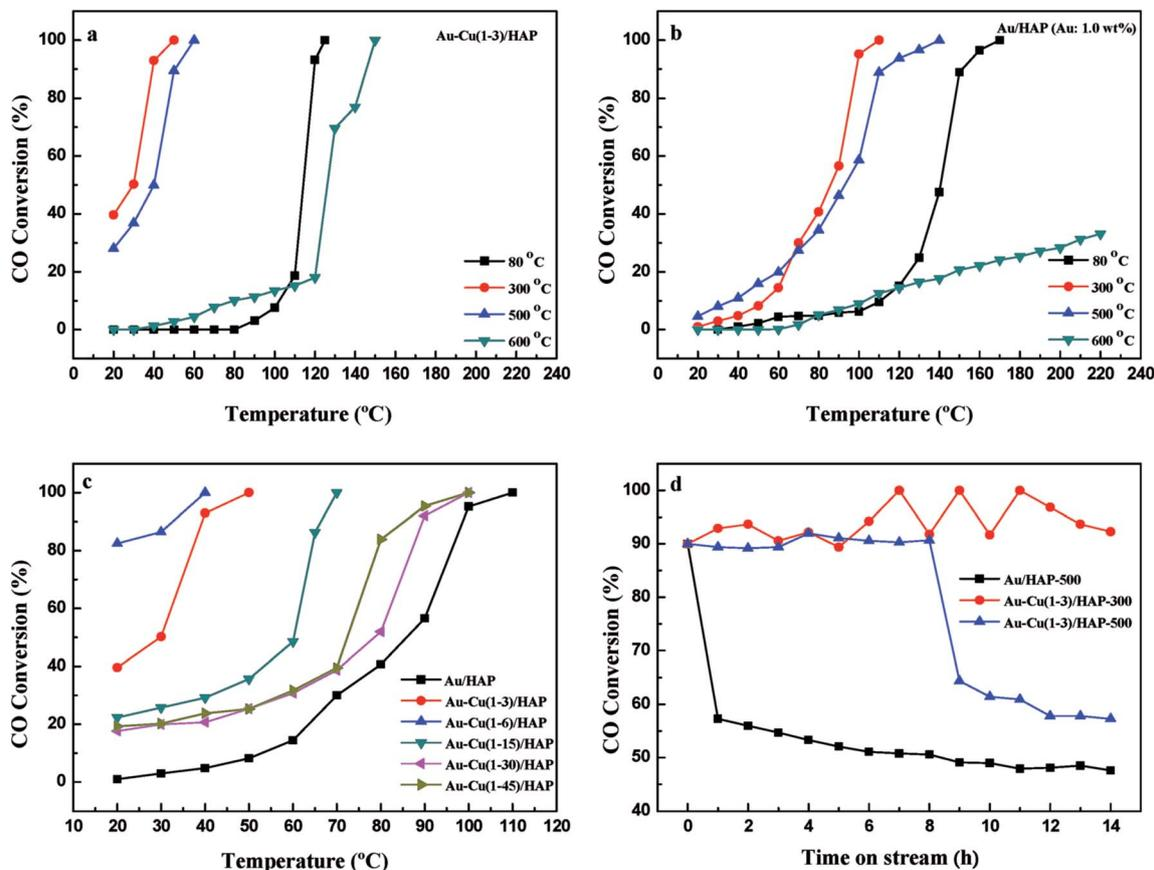
Fig. 12 Catalytic activity of Au–Cu(1–3)/HAP (Au: 1.0 wt%) (a) and Au/HAP (Au: 1.0 wt%) (b) calcined at different temperatures; Au–Cu/HAP catalysts with different Au : Cu atomic ratios (Au: 1.0 wt%) for CO oxidation (c); the stability of Au–Cu(1–3)/HAP (Au: 1.0 wt%) and Au/HAP (Au: 1.0 wt%) catalysts (d).
