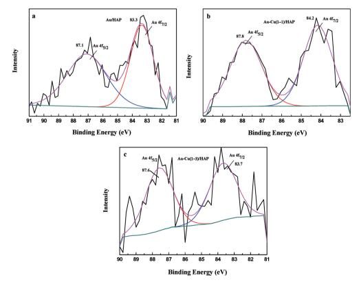
Fig. 6 Au 4f XPS spectra of Au/HAP (a), Au-Cu(1-1)/HAP (b) and Au-Cu(1-3)/HAP (c) (nominal total gold and copper loading: 2.0 wt%).
