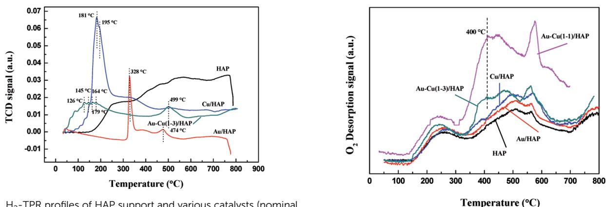
Fig. 9 H<sub>2</sub>-TPR profiles of HAP support and various catalysts (nominal total gold and copper loading: 2.0 wt%).
