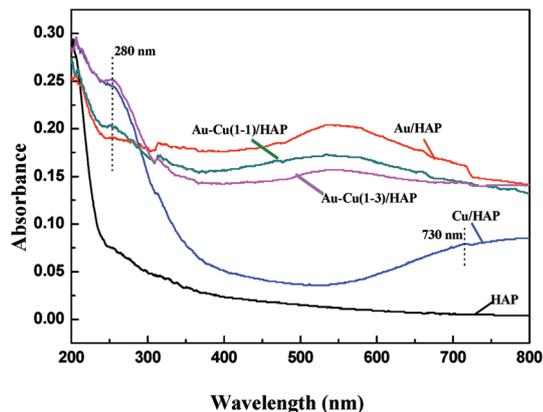
Fig. 5 UV-Vis DRS of HAP support and various catalysts (nominal total gold and copper loading: 2.0 wt%).
