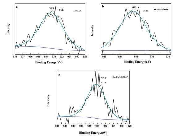
Fig. 7 Cu 2p<sub>3/2</sub> XPS spectra of Cu/HAP (a), Au-Cu(1-1)/HAP (b) and Au-Cu(1-3)/HAP (c) (nominal total gold and copper loading: 2.0 wt%).
