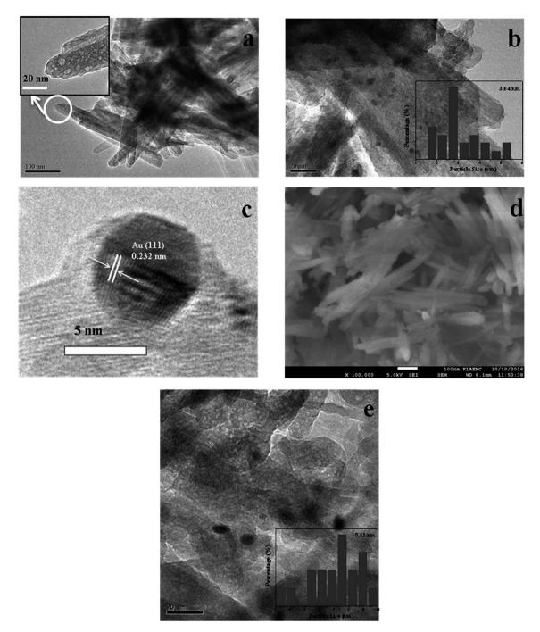
Fig. 2 TEM and SEM images of Au/HAP (Au: 2.0 wt%). TEM images (a, b), HR-TEM image (c), SEM image (d) and TEM image after reaction (e).
