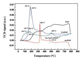
Fig. 9  $H_2$ -TPR profiles of HAP support and various catalysts (nominal total gold and copper loading: 2.0 wt%).
