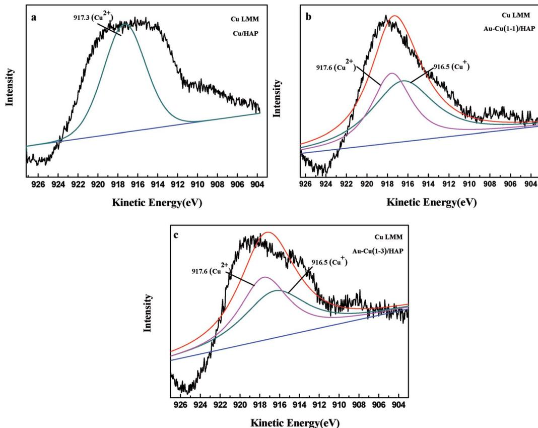
Fig. 8 Kinetic energy spectra of the Cu Auger LMM for Cu/HAP (a), Au–Cu(1–1)/HAP (b) and Au–Cu(1–3)/HAP (c) (nominal total gold and copper loading: 2.0 wt%).
