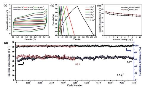
Fig. 15 (a) Cyclic voltammetry (CV) curves and (b) galvanostatic charge/discharge (GCD) curves of the  $RuO_2@C/rGO$ -based ASC. (c) Specific capacitances of the  $RuO_2@C/rGO$  and  $RuO_2/rGO$ -based ASC. (d) Cycling stability and coulombic efficiency of the  $RuO_2@C/rGO$ -based ASC. Reprinted with permission from ref. 118. Copyright 2016 Royal Society of Chemistry.
