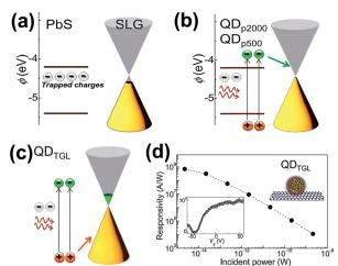
Fig. 8 Schematic illustration of the energy states (a) before depositing QDs on graphene, (b) after depositing QD $_{P2000}$  and QD $_{P500}$  on graphene and (c) after depositing QD $_{TGL}$  on graphene. (d) Photoresponsivity as a function of the incident light power of the QD $_{TGL}$ /GR transistor device. The bottom left inset shows photoresponsivity as a function of gate voltage ( $V_g$ ). Reprinted with an Open Access from ref. 59. Published by WILEY-VCH Verlag Gmbh & Co. KGaA, 2015.
