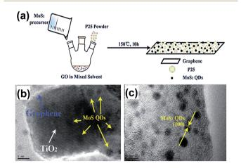
Fig. 4 (a) Schematic demonstration of the fabrication of the  $MoS_2$  QDs-graphene- $TiO_2$  composite. (b) HRTEM image of the  $MoS_2$  QDs-graphene- $TiO_2$  composite. (c) HRTEM image of the  $MoS_2$  QDs-graphene hybrid. Reprinted with permission from ref. 53. Copyright 2015 Royal Society of Chemistry.
