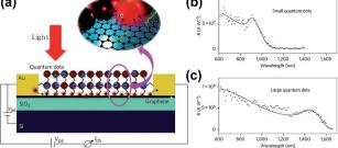
Fig. 13 (a) Schematic illustration of a phototransistor based on the PbS QDs/GR composite. Inset: photo-generated electrons and holes prefer to be transferred to graphene. Spectral responsivity of two devices based on small PbS QDs (b) and large PbS QDs (c). Reprinted with permission from ref. 63. Copyright 2012 Macmillan Publishers
