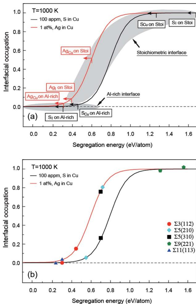
Fig. 5 Interfacial site occupation versus segregation energy for Ag and S. (a) interface (b) grain boundary as calculated from Mclean's equation for bulk concentrations of  $C_{Ag} = 1$  at% and  $C_S = 100$  appm, under  $T = 1000$  K.
