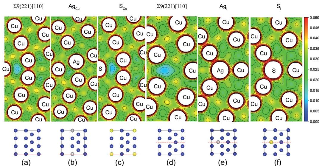
Fig. 4 Valence electron density contours of  $\Sigma 9(221)[110]$  GBs (in unit of  $e \text{ \AA}^{-3}$ ): (a) and (d) the clean GB, (b) substitutional Ag ( $Ag_{\text{Cu}}$ ), (c) substitutional S ( $S_{\text{Cu}}$ ), (e) interstitial Ag ( $Ag_{\text{I}}$ ), (f) interstitial S ( $S_{\text{I}}$ ).
