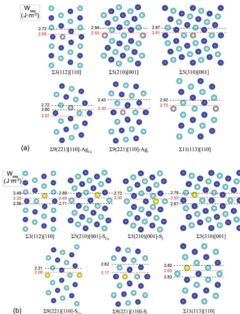
Fig. 3 Segregation structures and  $W_{\text{sep}}$  for Ag (a) and S (b) on low- $\Sigma$  STGBs ( $\Sigma \leq 11$ ) of Cu. Blue and cambridge blue spheres denote atoms on different  $\langle 110 \rangle$  planes for the  $\langle 110 \rangle$  tilt GBs and  $\langle 100 \rangle$  planes for the  $\langle 100 \rangle$  tilt GBs.
