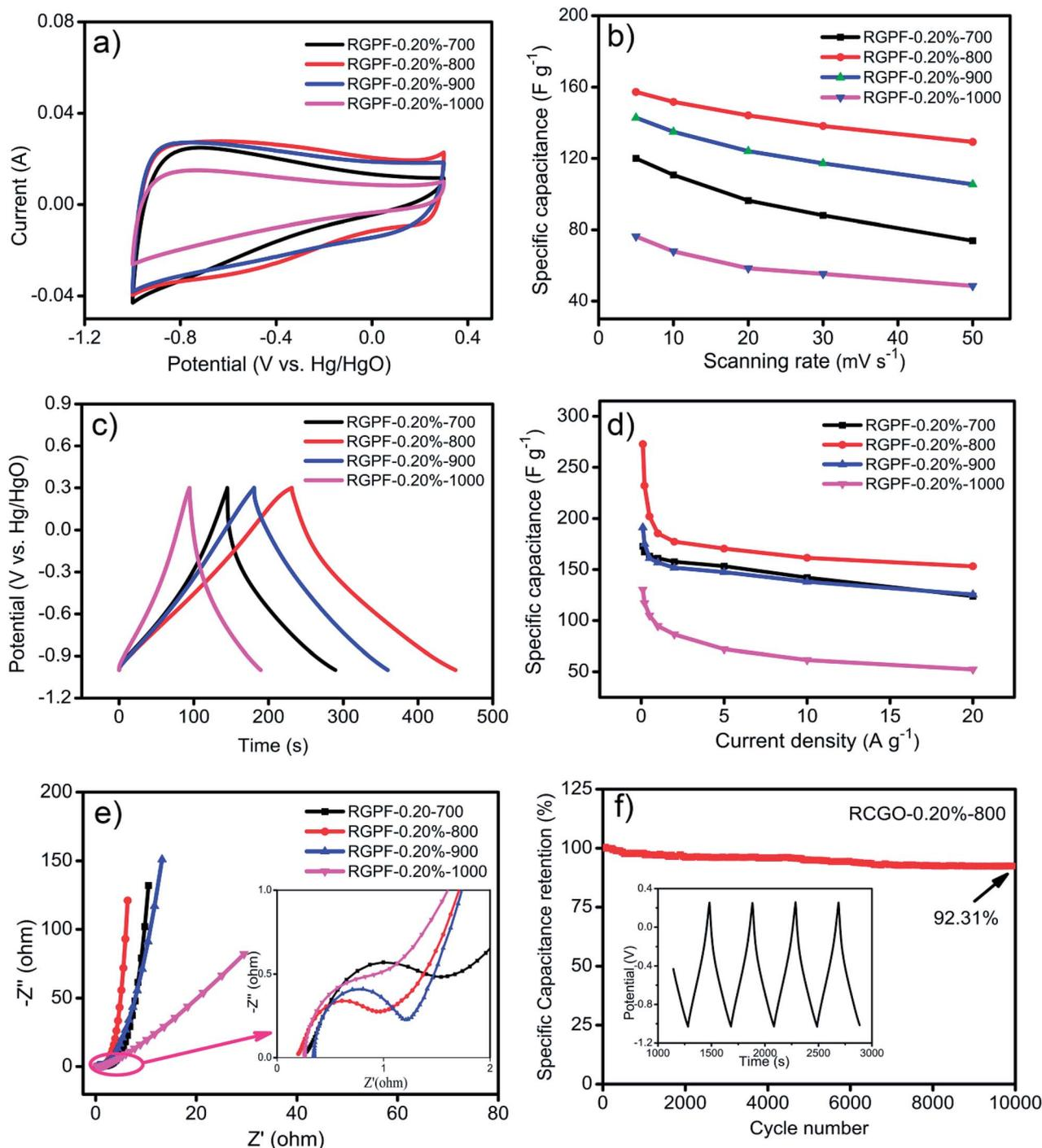
Fig. 5 (a) CV curves at  $20 \text{ mV s}^{-1}$ ; (b) specific capacitance from CV curves of as a function of scan rate; (c) CP curves at  $1 \text{ A g}^{-1}$ ; (d) specific capacitance from CP curves as a function of current density; (e) Nyquist plot from  $10 \text{ mHz}$  to  $100 \text{ kHz}$  for RGPF-0.20%- $t$ ; (f) capacitance retention of RGPF-0.20%-800 over  $10\,000$  cycles at  $1 \text{ A g}^{-1}$ , the inset is the typical measured CP curves.
