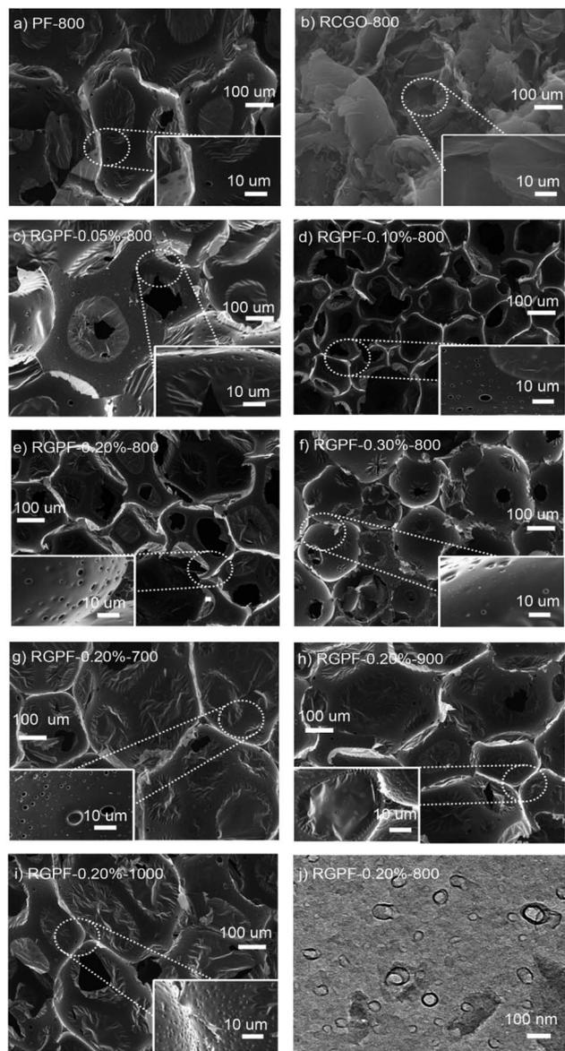
Fig. 3 (a–i) SEM images of the prepared materials, the insets are SEM images under high magnification; (j) TEM image of RGPF-0.20%-800.
