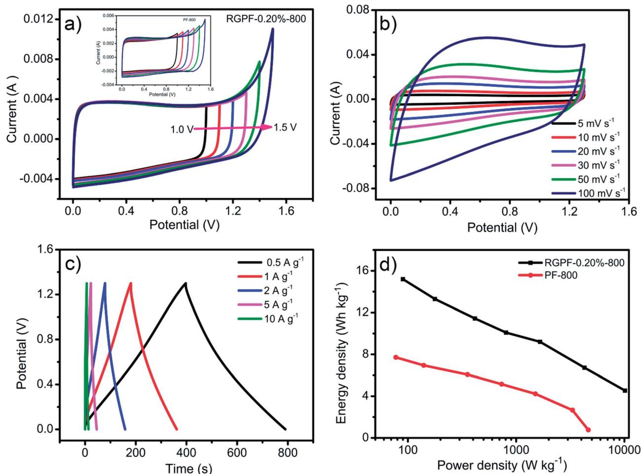
Fig. 6 (a) CV curves with different potential windows at  $5 \text{ mV s}^{-1}$ , (b) CV curves at different scan rates, (c) CP curves at different current density and (d) Ragone plots for RGPF-0.20%-800 and PF-800 in two-electrode system in 6 M KOH.
