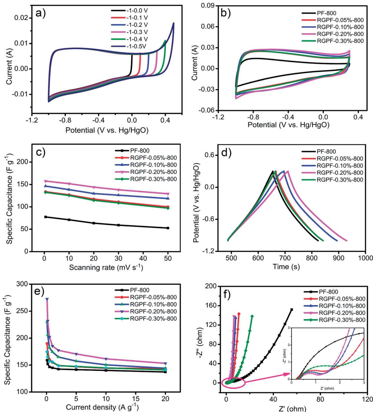
Fig. 4 (a) CV curves of the RGPF-0.02%-800 at  $5 \text{ mV s}^{-1}$  in different potential windows; (b) CV curves at  $20 \text{ mV s}^{-1}$ ; (c) specific capacitance from CV curves as a function of scan rate; (d) CP curves at  $1 \text{ A g}^{-1}$ ; (e) specific capacitance from CP curves as a function of current density; (f) Nyquist plots from 10 mHz to 100 kHz for PF-800 and RGPF-*m*-800.
