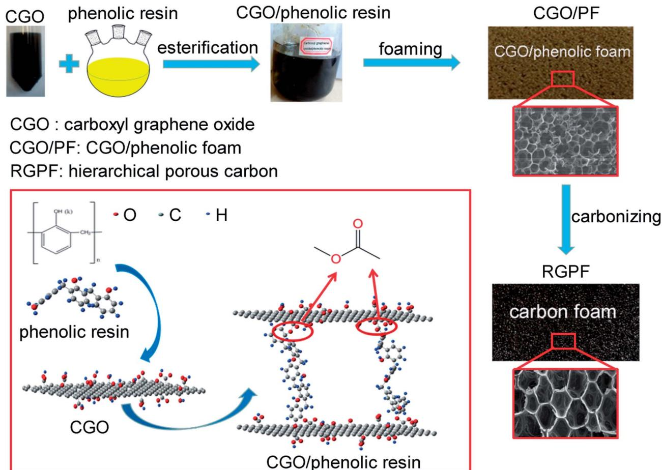
Scheme 1 Schematic illustration of the preparation of RGPF.
