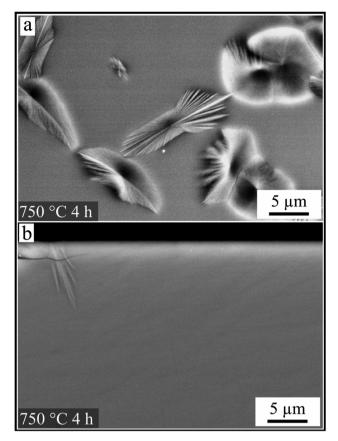
Fig. 6 Microstructures of a polished surface after a heat treatment at 750 °C for 4 h. Comparison of crystals observed in plane view (a) and corresponding cross section (b) at the same magnification.
