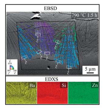
Fig. 8 SEM micrograph and combined EBSD-EDXS measurement of a cross section after crystallization for 1.5 h at 790  $^{\circ}$ C, stemming from an as-cut surface. The combined IQ and IPF map of the EBSD scan are superimposed onto the SEM micrograph to illustrate orientations relative to the image plane. Crystal orientation and c-axes are additionally marked. The black frame represents the scanned area. Lower part: simultaneously measured elemental analysis of the combined EBSD-EDXS scan.
