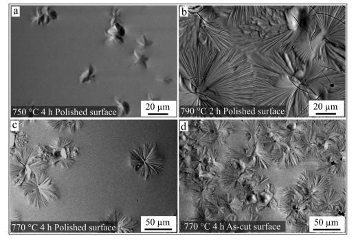
Fig. 5 SEM micrographs of samples heat-treated at different temperatures, and with surfaces having different pretreatments. (a) Polished surface heat treated at 750 °C for 4 h; (b) polished surface heat treated at 790 °C for 2 h; (c) polished surface heat treated at 770 °C for 4 h; (d) as-cut surface (compare with Fig. 2) heat treated at 770 °C for 4 h.
