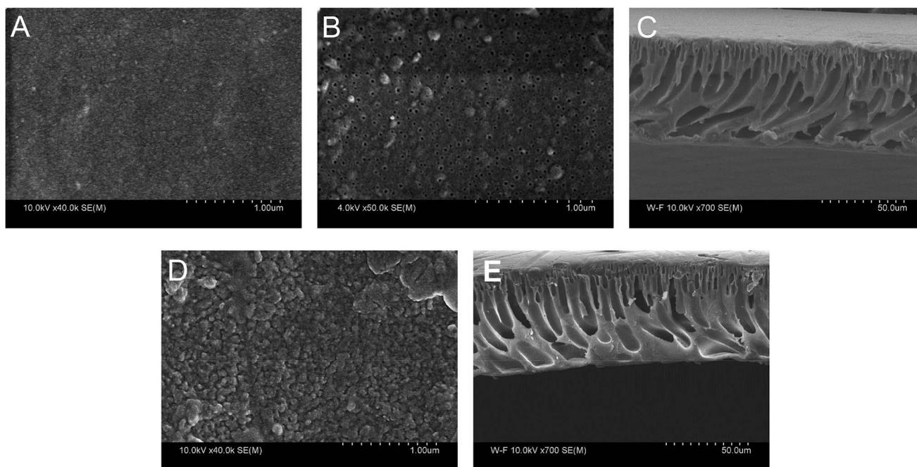
Fig. 10 Surface FE-SEM images of top surface (A), bottom surface (B), and cross-section (C) of PAN-COOH membrane, top surface (D), and cross-section (E) of PAN-[PAH/(PSS-TPPS)]<sub>6</sub> membrane (the bottom surface image of PAN-[PAH/(PSS-TPPS)]<sub>6</sub> membrane was not shown because no distinction compared with the substrate was observed).
