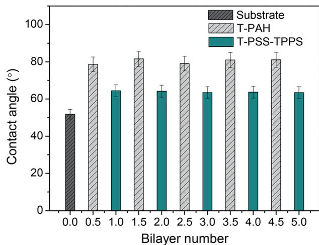
Fig. 9 Water contact angles of PAN-[PAH/(PSS-TPPS)]<sub>6</sub> membranes with different layers prepared at 0.5 M of salt and pH 6.5.
