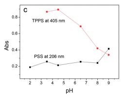
Fig. 1 DRUV spectra of PAN-[PAH/(PSS-TPPS)]<sub>6</sub> membranes prepared from PSS-TPPS solution at pH 6.5 and PAH solutions at different pH values (a, TPPS; b, PSS), and absorbance at 405 and 206 nm at different pH values of PAH (c). The absorbance at 405 nm at pH 2.0 of PAH was not displayed because TPPS formed J-aggregates here.
