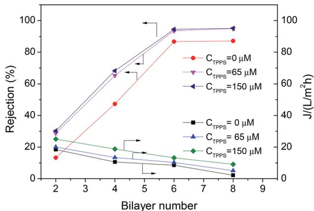
Fig. 11 Rejection properties of the PAN-(PAH/(PSS-TPPS))<sub>n</sub>/(PAH/PSS) membranes prepared with different TPPS initial concentrations. The concentration of feed MgSO<sub>4</sub> was 2.0 g L<sup>-1</sup>.
