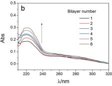
Fig. 7 DRUV spectra of PAN-[PAH/(PSS-TPPS)]<sub>n</sub> membranes with different number of bilayer (TPPS (a) and PSS (b)). The concentration of PAH, PSS, and TPPS were 1.0 g L<sup>-1</sup>, 1.0 g L<sup>-1</sup>, and 65  $\mu$ M, respectively. The pH value of solutions was 6.5 and ionic strength was 0.5 M.
