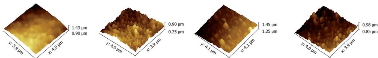
Fig. 2 AFM images of PAN support membrane (A); and PAN-[PAH/(PSS-TPPS)]<sub>6</sub> membranes prepared from PSS-TPPS solutions at pH 6.5 and PAH solutions at pH values of 2.0 (B), 4.5 (C), and 9.0 (D).
