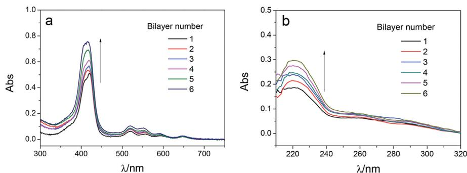
Fig. 7 DRUV spectra of PAN-[PAH/(PSS-TPPS)]<sub>n</sub> membranes with different number of bilayer (TPPS (a) and PSS (b)). The concentration of PAH, PSS, and TPPS were 1.0 g L<sup>-1</sup>, 1.0 g L<sup>-1</sup>, and 65 μM, respectively. The pH value of solutions was 6.5 and ionic strength was 0.5 M.
