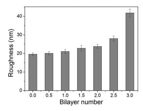
Fig. 8 Surface roughness of PAN-[PAH/(PSS-TPPS)] $_n$  membranes with different bilayer numbers prepared at 0.5 M ionic strength and pH 6.5. For example, n=2 means the membrane had 2 PAH/(PSS-TPPS) bilayers and the outmost layer (terminating layer) is PSS-TPPS; n=2.5 means the membrane had one more PAH coating (*i.e.*, half of a bilayer) in addition to the 2 PAH/(PSS-TPPS) bilayers, with PAH being the terminating layer.
