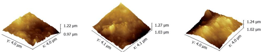
Fig. 4 AFM images of PAN-[PAH/(PSS-TPPS)]<sub>6</sub> membranes prepared from PAH solutions at pH 6.5 and PSS-TPPS solutions at pH values of 2.0 (A), 4.5 (B), and 8.0 (C).
