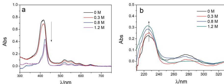
Fig. 5 DRUV spectra of PAN-[PAH/(PSS-TPPS)]<sub>6</sub> membranes prepared at different ionic strengths (TPPS (a) and PSS (b)).
