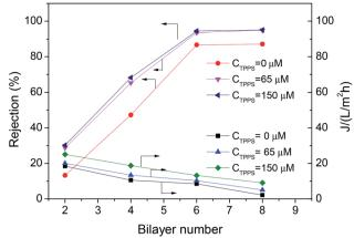
Fig. 11 Rejection properties of the PAN-(PAH/PSS-TPPS)<sub>p</sub>/(PAH/PSS) membranes prepared with different TPPS initial concentrations. The concentration of feed MgSO<sub>4</sub> was 2.0 g L<sup>-1</sup>
