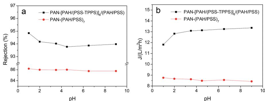
Fig. 12 Water flux and rejection of PAN-(PAH/PSS)<sub>7</sub> and PAN-[PAH/(PSS-TPPS)]<sub>6</sub>/(PAH/PSS) membranes at different pH values.
