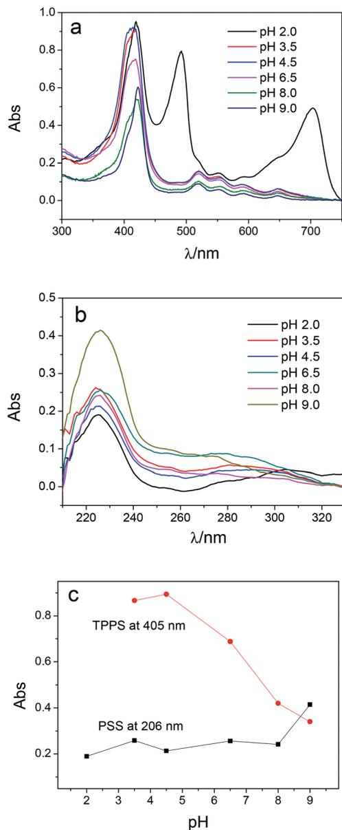
Fig. 1 DRUV spectra of PAN-[PAH/(PSS-TPPS)]<sub>6</sub> membranes prepared from PSS-TPPS solution at pH 6.5 and PAH solutions at different pH values (a, TPPS; b, PSS), and absorbance at 405 and 206 nm at different pH values of PAH (c). The absorbance at 405 nm at pH 2.0 of PAH was not displayed because TPPS formed J-aggregates here.
