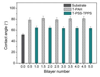
Fig. 9 Water contact angles of PAN-[PAH/(PSS-TPPS)] $_{\rm 6}$  membranes with different layers prepared at 0.5 M of salt and pH 6.5.
