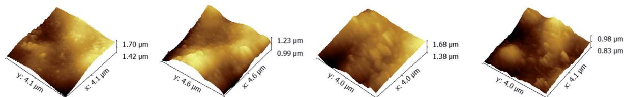
Fig. 6 AFM images of PAN-[PAH/(PSS-TPPS)]<sub>6</sub> membranes prepared at different ionic strengths (0 (A), 0.3 (B), 0.8 (C), and 1.2 (D)).
