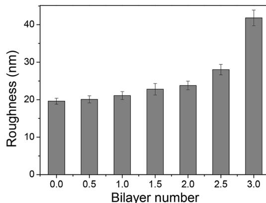
Fig. 8 Surface roughness of PAN-[PAH/(PSS-TPPS)]<sub>n</sub> membranes with different bilayer numbers prepared at 0.5 M ionic strength and pH 6.5. For example,  $n = 2$  means the membrane had 2 PAH/(PSS-TPPS) bilayers and the outmost layer (terminating layer) is PSS-TPPS;  $n = 2.5$  means the membrane had one more PAH coating (*i.e.*, half of a bilayer) in addition to the 2 PAH/(PSS-TPPS) bilayers, with PAH being the terminating layer.
