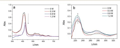
Fig. 5 DRUV spectra of PAN-[PAH/(PSS-TPPS)]<sub>6</sub> membranes prepared at different ionic strengths (TPPS (a) and PSS (b)).
