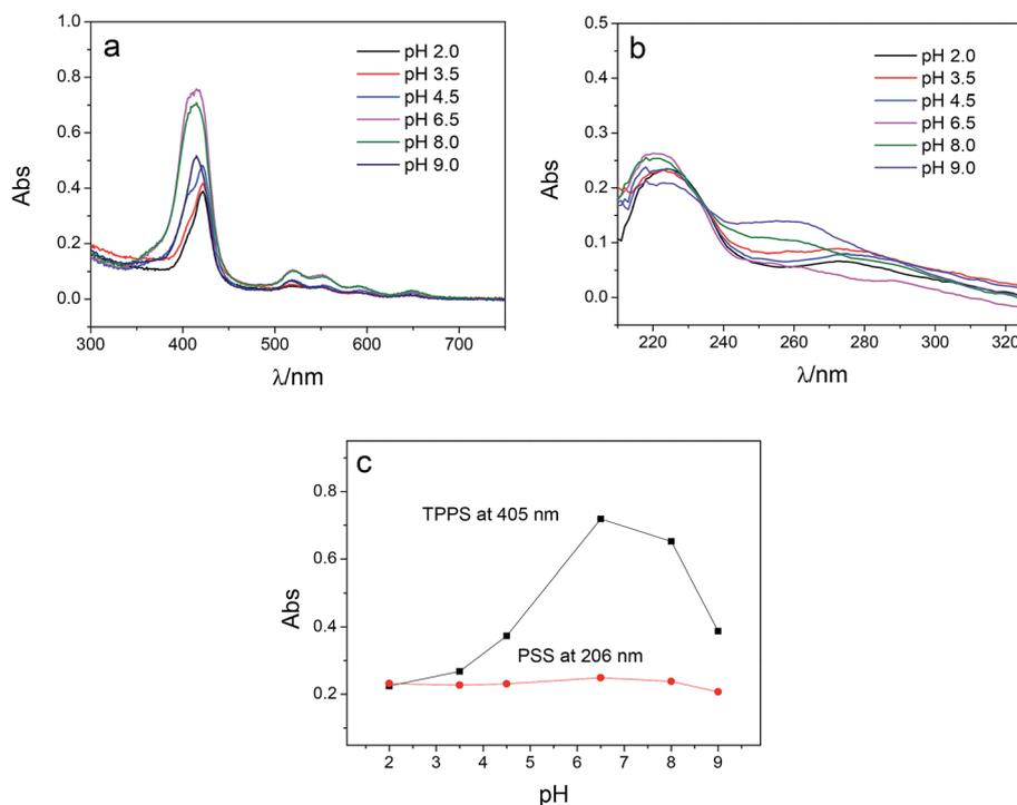
Fig. 3 DRUV spectra of PAN-[PAH/(PSS-TPPS)]<sub>6</sub> membranes prepared from PAH solutions at pH 6.5 and PSS-TPPS solutions at different pH values (a, TPPS; b, PSS), and absorbance at 405 and 206 nm at different pH values of PSS (c).
