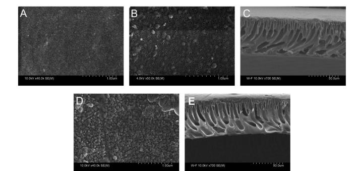
Fig. 10 Surface FE-SEM images of top surface (A), bottom surface (B), and cross-section (C) of PAN-COOH membrane, top surface (D), and cross-section (E) of PAN-[PAH/(PSS-TPPS)]<sub>6</sub> membrane (the bottom surface image of PAN-[PAH/(PSS-TPPS)]<sub>6</sub> membrane was not shown because no distinction compared with the substrate was observed).
