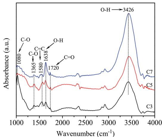
Fig. 1 FTIR spectrum of carboxyl-functionalized multi-walled carbon nanotubes.
