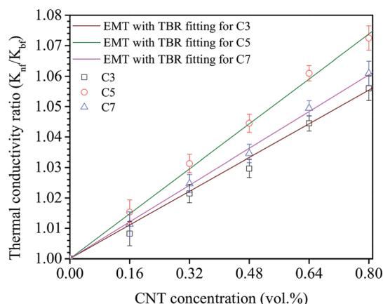
Fig. 7 Comparison of experimental results with the effective medium theory incorporated the thermal boundary resistances.
