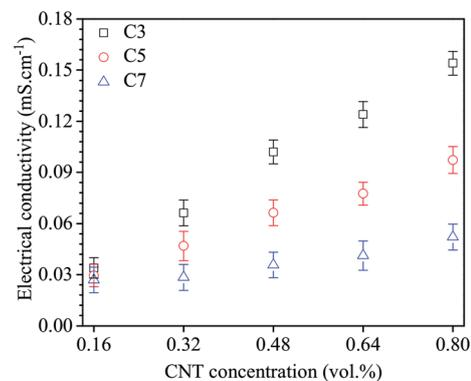
Fig. 5 Electrical conductivity of nanofluids versus CNT concentrations.
