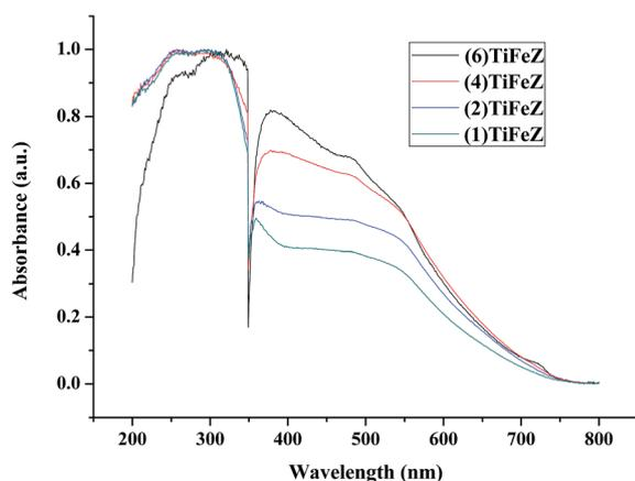
Fig. 3 UV-vis diffuse reflectance spectra of (n)TiFeZ.
