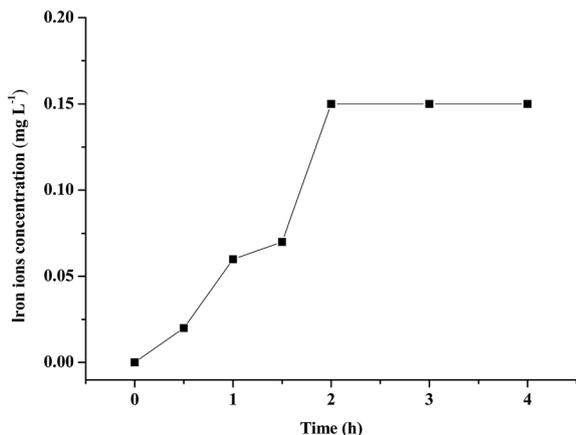
Fig. 7 Iron ion concentration in water during CIP degradation by (n)TiFeZ.
