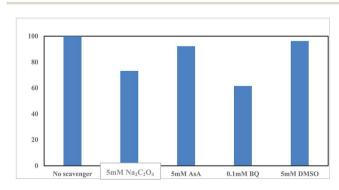
Fig. 9 Effect of reactive radical scavengers on CIP degradation by (n) TiFeZ-PS after 3 h (CIP concentration, 500 mg L<sup>-1</sup>; dosage of catalyst, 1 g L<sup>-1</sup>; and pH, 7.0).
