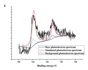
Fig. 8 Fe 2p core level photoelectron spectra of (n)TiFeZ before (A) and after (B) CIP degradation.
