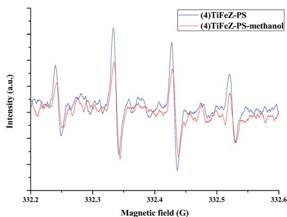
Fig. 11 EPR spectra versus time for supernatant of  $(4)\text{TiFeZ-PS-CIP}$  batch experiment ( $[\text{PS}] = 5.0 \text{ mM}$ ,  $[(n)\text{TiFeZ}] = 1 \text{ g L}^{-1}$ ,  $[\text{DMPO}] = 10 \text{ mM}$ , and  $\text{pH} = 7.0$ ).
