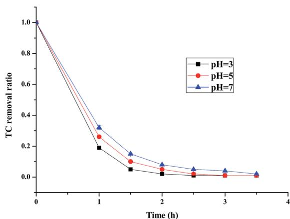
Fig. 6 Effects of pH on the degradation of CIP (CIP concentration, 500 mg L<sup>-1</sup>; dosage of catalyst, 1 g L<sup>-1</sup>).
