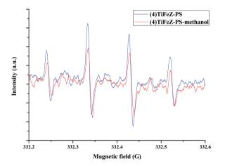
Fig. 11 EPR spectra *versus* time for supernatant of (4)TiFeZ-PS-CIP batch experiment ([PS] = 5.0 mM, [(n)TiFeZ] = 1 g L<sup>-1</sup>, [DMPO] = 10 mM, and pH = 7.0).
