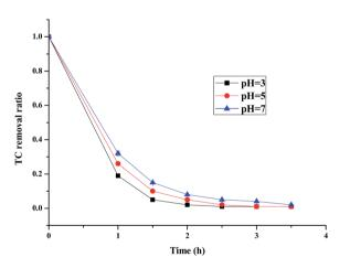
Fig. 6 Effects of pH on the degradation of CIP (CIP concentration, 500 mg  $\rm L^{-1}$ ; dosage of catalyst, 1 g  $\rm L^{-1}$ ).
