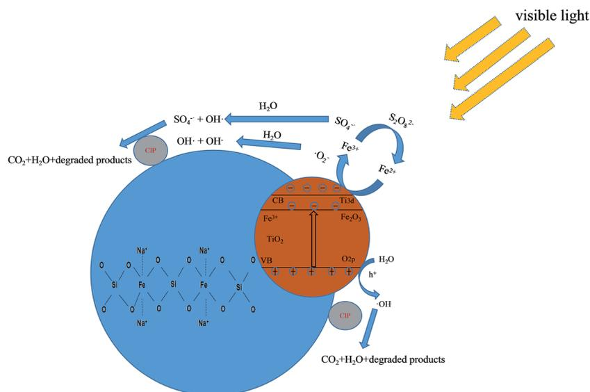
Fig. 12 Schematic of mechanisms of CIP degradation process by  $(n)\text{TiFeZ-PS}$ .
