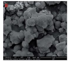
Fig. 2 FESEM images of (A) zeolite X and (B) (4)TiFeZ
