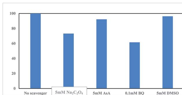
Fig. 9 Effect of reactive radical scavengers on CIP degradation by (n)TiFeZ-PS after 3 h (CIP concentration, 500 mg L<sup>-1</sup>; dosage of catalyst, 1 g L<sup>-1</sup>; and pH, 7.0).
