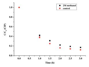
Fig. 10 Effects of methanol on CIP degradation by the (n)TiFeZ-PS system ([PS] = 5.0 mM, [(n)TiFeZ] = 1 q L<sup>-1</sup>, and pH = 7.0).
