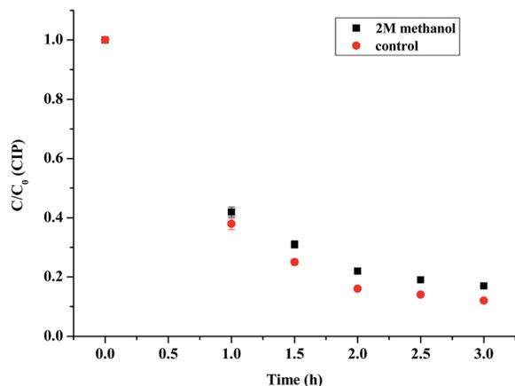
Fig. 10 Effects of methanol on CIP degradation by the  $(n)\text{TiFeZ-PS}$  system ( $[\text{PS}] = 5.0 \text{ mM}$ ,  $[(n)\text{TiFeZ}] = 1 \text{ g L}^{-1}$ , and  $\text{pH} = 7.0$ ).
