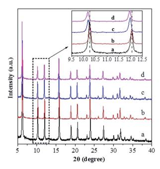
Fig. 1 XRD patterns for the unmodified and modified USY zeolite catalysts: (a) USY; (b) USY-acid; (c) Ni-USY-acid; (d) ZnCl<sub>2</sub>/Ni-USY-acid (the inset is the enlargement of the patterns for  $2\theta = 9.5-12.5^{\circ}$ ).
