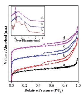
Fig. 3 N<sub>2</sub>-adsorption/desorption isotherms and BJH pore-size distribution curves for the unmodified and modified USY zeolite catalysts: (a) USY; (b) USY-acid; (c) Ni-USY-acid; (d) ZnCl<sub>2</sub>/Ni-USYacid.
