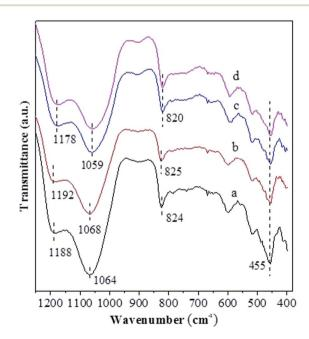
Fig. 2 FT-IR spectra for the unmodified and modified USY zeolite catalysts: (a) USY; (b) USY-acid; (c) Ni-USY-acid; (d) ZnCl<sub>2</sub>/Ni-USYacid.
