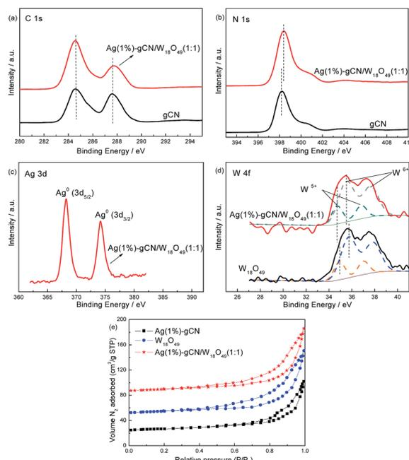
Fig. 3 XPS spectra (a–d) and  $\text{N}_2$  adsorption (e) of gCN,  $\text{W}_{18}\text{O}_{49}$  and Ag(1%)-gCN/ $\text{W}_{18}\text{O}_{49}$ (1 : 1).
