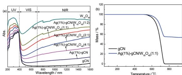
Fig. 2 Powder absorbance spectra of as-prepared samples from UV to near infrared region (a) and TG analysis (b).
