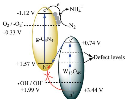
Fig. 8 The possible Z-scheme mechanism over  $Ag(1\%)-gCN/W_{18}O_{49}(1:1)$ .
