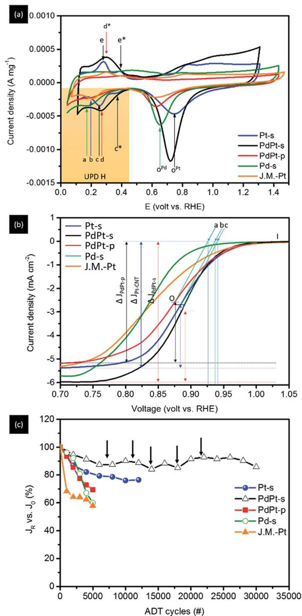
Fig. 5 (a) CV, (b) LSV, and (c) ADT curves of experimental Pt-s, PdPt-s, PdPt-p, Pd-s NPs, and commercial Pt catalysts (J.M.-Pt). In CV curve of Pt-s, current peaks c and c\* in negative sweep curve refer to adsorption responses of H<sup>+</sup> at (111) and (200) facets of metallic Pt. The significant higher current density of peak c reveals the preferential grow of (111) facets in Pt-s. The counterpart responses of H<sup>+</sup> desorption appears at peaks e and e\* in positive sweep curve.
