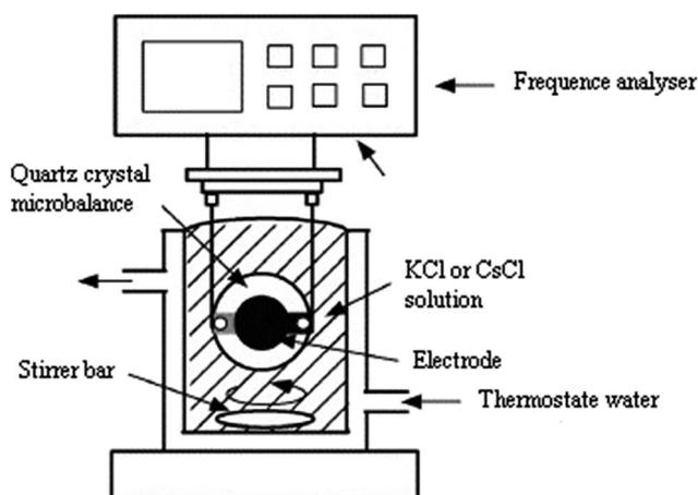
Fig. 3 Experimental setup for adsorption measurements with QCM.
