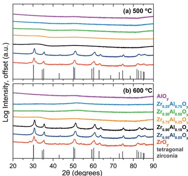
Fig. 3 GIXRD of single-coat ZAO films annealed at (a) 500 °C and (b) 600 °C. The tetragonal zirconia phase (ICSD 66781)<sup>69</sup> is plotted for reference.
