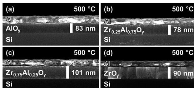
Fig. 5 SEM cross-sectional images of two-coat (a)  $\text{ZrO}_y$ , (b)  $\text{Zr}_{0.75}\text{Al}_{0.25}\text{O}_y$ , (c)  $\text{Zr}_{0.50}\text{Al}_{0.50}\text{O}_y$ , and (d)  $\text{AlO}_y$  films annealed at  $500\text{ }^\circ\text{C}$ .
