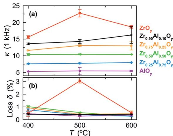
Fig. 6 (a) Dielectric constants ( $\kappa$ ) measured at 1 kHz and (b) corresponding loss tangents (loss  $\delta$ ) for MIS devices fabricated from two-coat ( $\sim 100\ \text{nm}$ ) ZAO films annealed at various temperatures. Error bars were determined using measurements taken from three separate batches of ZAO-based MIS devices. A plot of  $\kappa$  and loss  $\delta$  as a function of frequency for ZAO-based MIS devices fabricated at  $500\text{ }^\circ\text{C}$  can be found in Fig. S4.†
