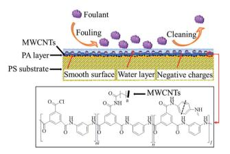
Fig. 12 Antifouling mechanism of mixed-matrix RO membranes.
