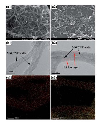
Fig. 4 SEM images of (a1) raw MWCNTs and (a2) MWCNT-COOH; TEM images of (b1) MWCNT-COOH and (b2) PAAm-6h; HAADF-STEM-EDS merged elemental mapping images of (c1) MWCNT-COOH and (c2) PAAm-6h. (C-red, N-blue and O-yellow).
