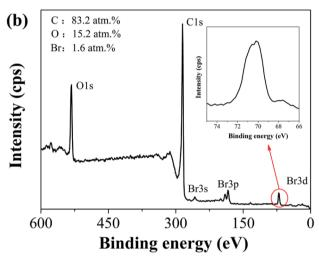
Fig. 2 (a) FTIR spectra of raw MWCNTs and functionalized MWCNTs; (b) XPS survey spectrum of MWCNT-Br, inset is enlarged image of Br 3d.
