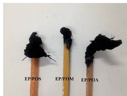
Fig. 8 Digital photos of char residue of EP/PPDA composites after LOI tests.
