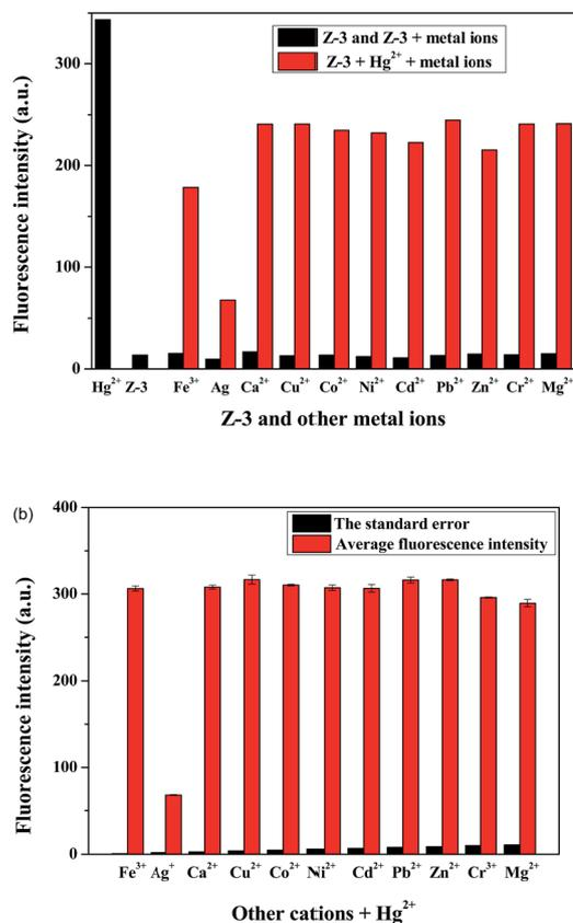
Fig. 2 (a) Fluorescence spectra of Z-3 and Z-3 +  $\text{Hg}^{2+}$  in the presence of 10 equiv. various metal ions in DMSO/ $\text{H}_2\text{O}$  (v/v, 3 : 2; buffered with HEPES, pH = 7.20) solutions; (b) error bar of Z-3 +  $\text{Hg}^{2+}$  in the presence of various cations.
