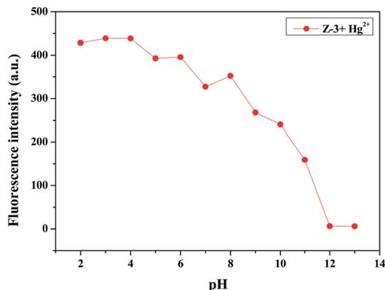
Fig. 4 Fluorescence intensity ( $\lambda_{\text{ex}} = 400$  nm and  $\lambda_{\text{em}} = 496$  nm) of the Z-3 + Hg<sup>2+</sup> complex at various pH values in DMSO/H<sub>2</sub>O (v/v, 3 : 2; buffered with HEPES, pH = 7.20) solution.
