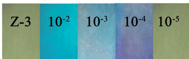
Fig. 5 Photographs of test strips (the concentration of Hg<sup>2+</sup> is 0 M,  $10^{-1}$  M,  $10^{-2}$  M,  $10^{-3}$  M,  $10^{-4}$  M,  $10^{-5}$  M, both under an UV lamp at 365 nm).
