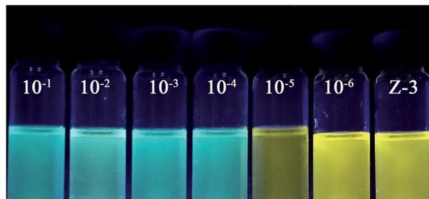
Fig. 6 Naked-eyes detection limit under UV lamp at 365 nm. From left to right, the concentration of Hg<sup>2+</sup> is  $10^{-1}$  M,  $10^{-2}$  M,  $10^{-3}$  M,  $10^{-4}$  M,  $10^{-5}$  M,  $10^{-6}$  and 0 M.
