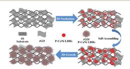
Fig. 5 The proposed growth process of the rGO/P-CoNi LDHs.
