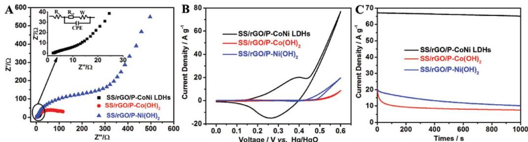
Fig. 9 The EIS plots (A), CV curves at scan rate of  $10 \text{ mV s}^{-1}$  (B) and CA curves at  $0.6 \text{ V}$  (C) of SS/rGO/P-CoNi LDHs (black), SS/rGO/P-Co(OH)<sub>2</sub> (red) and SS/rGO/P-Ni(OH)<sub>2</sub> (blue).
