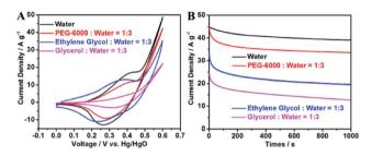
Fig. 7 CV curves (A) at scan rate of 10 mV s $^{-1}$  and CA curves (B) at 0.6 V of SS/P-CoNi LDHs in 1 M KOH electrolyte with 0.5 M methanol. The SS/P-CoNi LDHs were deposited in different alcohol–water component solvent.
