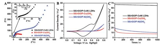
Fig. 9 The EIS plots (A), CV curves at scan rate of 10 mV s $^{-1}$  (B) and CA curves at 0.6 V (C) of SS/rGO/P-CoNi LDHs (black), SS/rGO/P-Co(OH) $_2$  (red) and SS/rGO/P-Ni(OH) $_2$  (blue).
