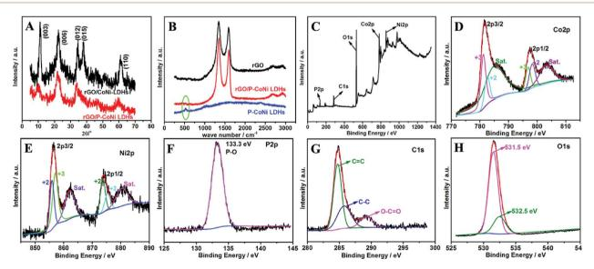
Fig. 2 (A) is the XRD pattern of rGO/CoNi LDHs (black curve) and rGO/P-CoNi LDHs (red curve). (B) is the Raman spectra of rGO (black curve), rGO/P-CoNi LDHs (red curve) and P-CoNi LDHs (blue curve). (C)-(H) are the XPS survey (C), Co 2p (D), Ni 2p (E), P 2p (F), C 1s (G) and O 1s (H) spectra of rGO/P-CoNi LDHs.
