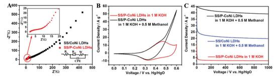
Fig. 6 (A) is the EIS plots of SS/P-CoNi LDHs and SS/CoNi LDHs in 1 M KOH with 0.5 M methanol. (B) is the CV curves of SS/P-CoNi LDHs in 1 M KOH electrolyte with (black) and without (red) 0.5 M methanol at scan rate of 10 mV s<sup>-1</sup>. (C) is the CA curves of SS/P-CoNi LDHs and SS/CoNi LDHs in 1 M KOH with and without 0.5 M methanol at 0.6 V.
