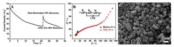
Fig. 10 (A) is the long-term CA curves of the SS/rGO/P-CoNi LDHs, (B) is the EIS plots of SS/rGO/P-CoNi LDHs before and after long-term CA measurement, (C) is the SEM image of SS/rGO/P-CoNi LDHs after long-term CA measurements.
