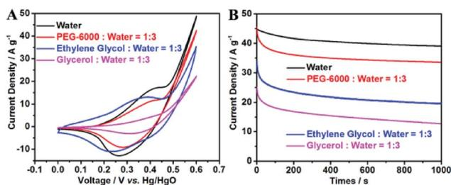
Fig. 7 CV curves (A) at scan rate of  $10 \text{ mV s}^{-1}$  and CA curves (B) at 0.6 V of SS/P-CoNi LDHs in 1 M KOH electrolyte with 0.5 M methanol. The SS/P-CoNi LDHs were deposited in different alcohol-water component solvent.
