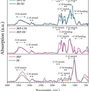
Fig. 7 FTIR spectra of wood sawdust samples and CM and HC obtained from them
