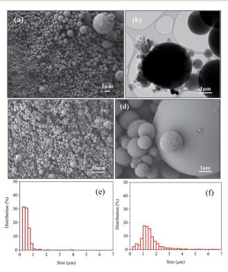
Fig. 3 Morphology of JRP-CM and JB-CM. (a, b and e) SEM, TEM images, and size distribution of JRP-CM, respectively, and (c, d and f) SEM images and size distribution of JB-CM.
