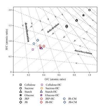
**Fig. 6** H/C *versus* O/C van Krevelen diagram of different carbohydrates, HC resulting from HTC of carbohydrates, <sup>17</sup> wood sawdust samples, and CM and HC obtained from them.
