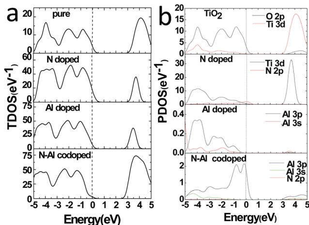
Fig. 3 TDOS (a) and PDOS (b) were calculated by the GGA + U method and plotted for pure  $\text{TiO}_2$ , N monodoped, Al monodoped, and N–Al codoped anatase  $\text{TiO}_2$ . The Fermi level of these systems is displayed with a gray dashed line.
