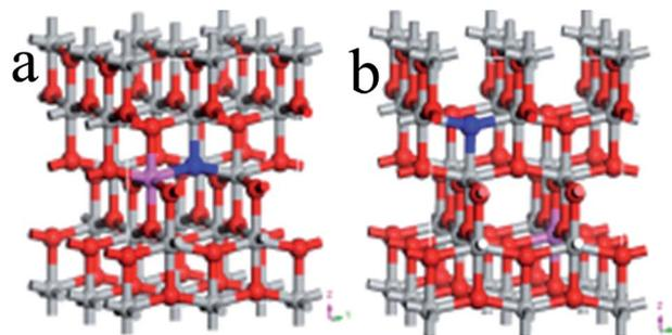
Fig. 1 Perspective view of the 2 × 2 × 1 supercell of N–Al codoped anatase TiO<sub>2</sub>, in which N and Al are next to each other (a) and far away (b). The red, gray, pink, and blue spheres represent O, Ti, Al, and N atoms, respectively.
