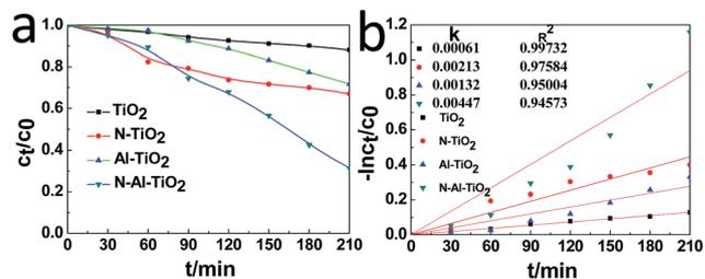
Fig. 6 (a) Photocatalytic degradation of MO by different catalysts and (b) the kinetics of the photocatalytic degradation of MO by them under the simulated visible light irradiation.
