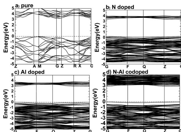
Fig. 2 The band structures for (a) pure  $TiO_2$ , (b) N monodoped, (c) Al monodoped, and (d) N-Al codoped anatase  $TiO_2$  calculated by the GGA + U method along the high symmetry lines of Brillouin zone. The dashed lines represent the Fermi level  $E_f$ .
