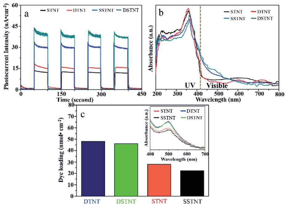
Fig. 5 (a)  $j-t$  curves upon chopped simulated solar light illumination at 0.3 V vs. Ag/AgCl reference electrode, (b) UV-visible absorption spectra and (c) dye loading measurements of annealed double and single walled TiO<sub>2</sub> nanotube arrays with and without hydrothermal treatment.
