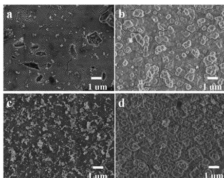
Fig. 8 SEM images for the samples of (a) STNT, (b) SSTNT, (c) DTNT and (d) DSTNT after soaking in SBF for 18 days.
