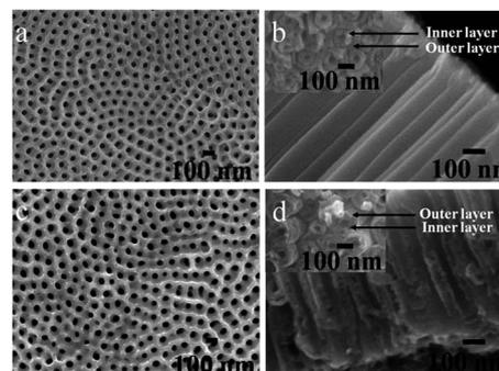
Fig. 1 SEM images of (a, b) as-anodized TiO<sub>2</sub> nanotube arrays (DTNT) and (c, d) SrTiO<sub>3</sub>/TiO<sub>2</sub> nanotube arrays (DSTNT) with double layer walled structure.
