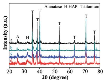
Fig. 7 XRD patterns of annealed double and single layer walled  $\text{TiO}_2$  nanotube arrays with and without hydrothermal treatment after soaking in SBF for 18 days. (a) STNT, (b) DTNT, (c) SSTNT and (d) DSTNT.
