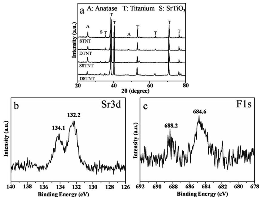
Fig. 4 (a) XRD patterns of annealed double and single layer walled  $\text{TiO}_2$  nanotube arrays with and without hydrothermal treatment; (b) and (c) high resolution XPS profiles of Sr 3d and F 1s of annealed double layer walled  $\text{TiO}_2$  nanotube arrays with hydrothermal treatment.
